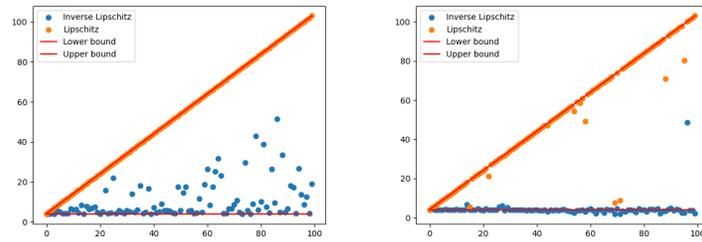
Figure 11: Estimated Lipschitz and inverse Lipschitz constants of BLNN with gradient descent with ReLU activation functions. The left figure is with 3 hidden layers and the right with 10. The  $x$  axis corresponds to  $j$  with  $\beta = 0.05 + 99.95 \cdot j/100$
