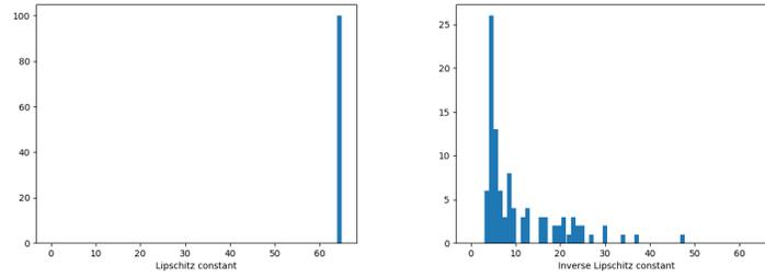
Figure 12: Histograms of Lipschitz and inverse Lipschitz constants of 100 (4, 60)-BLNNs with non-negative weights  $W_i^{(z)}$  initialized following the uniform distribution of [Glorot and Bengio \(2010\)](#). Negative elements were clamped to 0.
