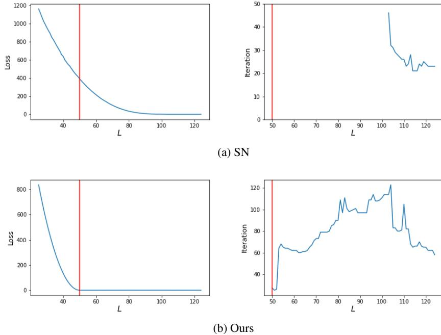
Figure 20: Results of fitting the linear function  $y = 50x$  with different  $L$  for SN and our model. The left figure is the loss in function of  $L$ , and the right figure is the first iteration that the loss was below 0.5 for each  $L$  (if there is no point, it means that a loss below 0.5 was never reached for this value of  $L$ ). The red line emphasizes the point of  $L = 50$ .
