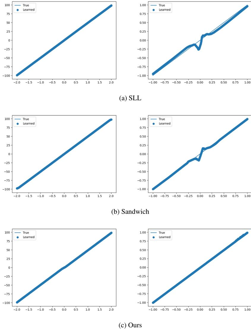
Figure 17: Results of fitting a linear function ( $y = 50x$  for left column and  $y = x$  for right column) with SLL (first), Sandwich (second row) and our method (third row) with a specified Lipschitzness of 50.
