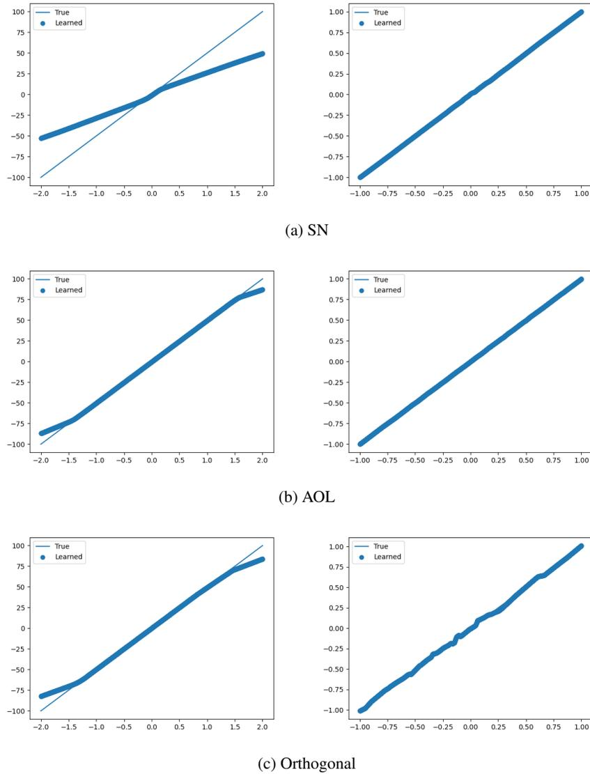
Figure 16: Results of fitting a linear function ( $y = 50x$  for left column and  $y = x$  for right column) with SN (first row), AOL (second row) and Orthogonal (third row) with a specified Lipschitzness of 50.
