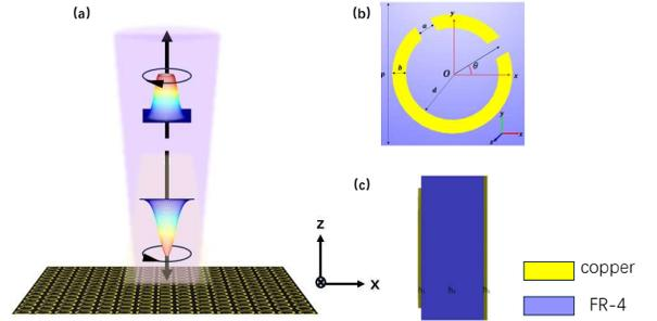
**Fig. 1.** (a) Schematic diagram of the reflected MS: The reflected CP wave carries OAM is consistent with the polarization state of the incident CP wave; (b) Top view of unit cell; (c) Side view of unit cell
