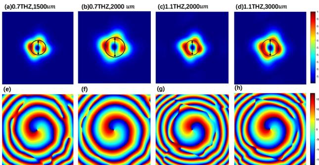
**Fig. 8.** The normalized reflection amplitudes:(a)  $L = 1500\mu\text{m}$  at  $f = 0.7\text{THz}$ , (b)  $L = 2000\mu\text{m}$  at  $f = 0.7\text{THz}$ , (c)  $L = 2000\mu\text{m}$  at  $f = 1.1\text{THz}$ , (d)  $L = 3000\mu\text{m}$  at  $f = 1.1\text{THz}$ ; Reflection phase: (e), (f), (g), and (h) correspond to (a), (b), (c), and (d), respectively.
