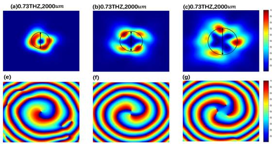
**Fig. 11.** The normalized reflection amplitudes at  $L = 2000\mu\text{m}$  are presented for three different topological charges: (a)  $l = +1$ , (b)  $l = +2$ , (c)  $l = +3$ . The corresponding reflection phases for (a), (b), (c) are shown in (d), (e), (f), respectively.
