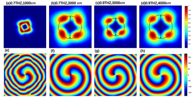
**Fig. 9.** The normalized reflection amplitudes are presented for the following conditions: (a)  $l = -2$  with  $L = 1000\mu\text{m}$  at  $f = 0.7\text{THz}$ , (b)  $l = -2$  with  $L = 3000\mu\text{m}$  at  $f = 0.7\text{THz}$ , (c)  $l = -2$  with  $L = 3000\mu\text{m}$  at  $f = 0.9\text{THz}$ , and (d)  $l = -2$  with  $L = 4000\mu\text{m}$  at  $f = 0.9\text{THz}$ . The corresponding reflection phases for (a), (b), (c), and (d) are shown in (e), (f), (g), and (h), respectively.
