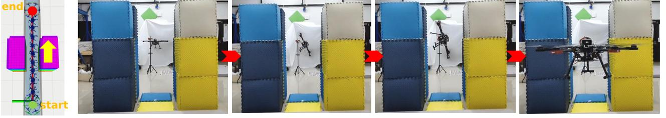
Fig. 8. OmniHex executes the generated trajectory to fly through a narrow passage. The leftmost figure is the visualization of the generated trajectory, and the others are snapshots of the experiment. The red arrow indicates the chronological order of the snapshots.
