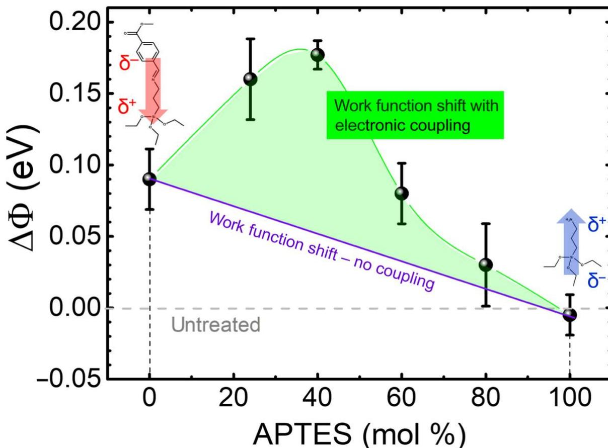
**Fig. 4. Work function shift in substrates treated with mixed SAMs.** Dependence of the work function shift of the  $\text{SiO}_2$  substrate on the CMPTM/APTES ratio. The purple line represents the estimated shift in the absence of CT between the two SAMs. The internal molecular dipoles are indicated in red and blue, respectively.
