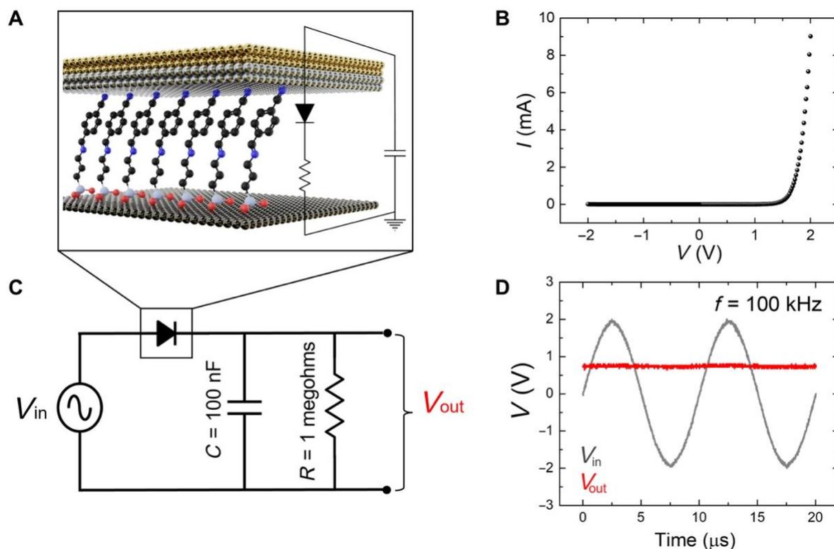
**Fig. 7. Basic circuits with molecular rectifiers consisting of mixed SAMs.** (A) Cross-sectional schematic of the molecular rectifiers. (B) Typical current-voltage characteristics of the molecular rectifiers. (C) AC/DC rectifier circuit diagram. (D) Input and output voltages corresponding to the circuit presented in (C).
