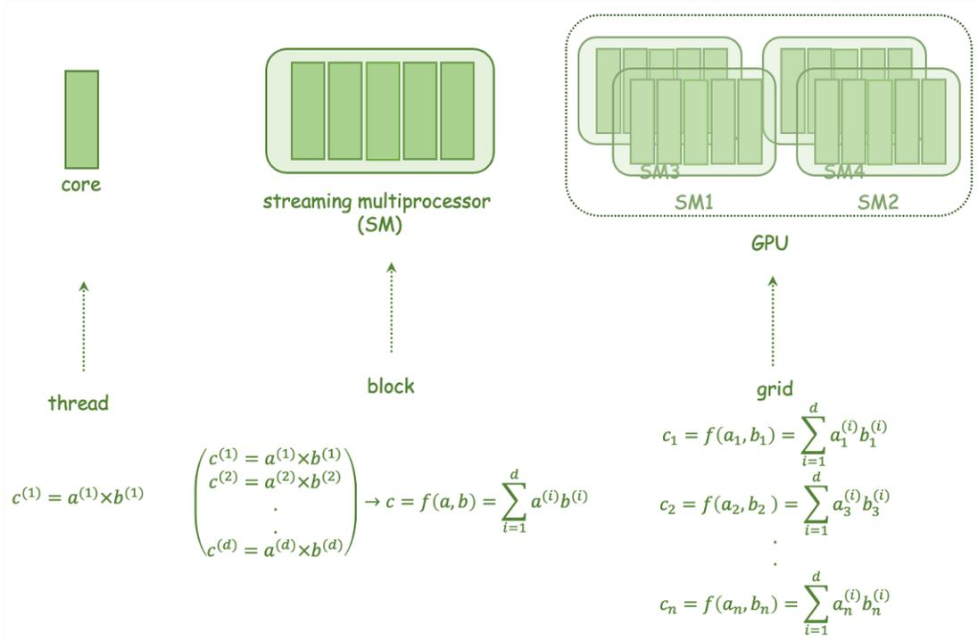
**Figure 1 GPU Architecture**
