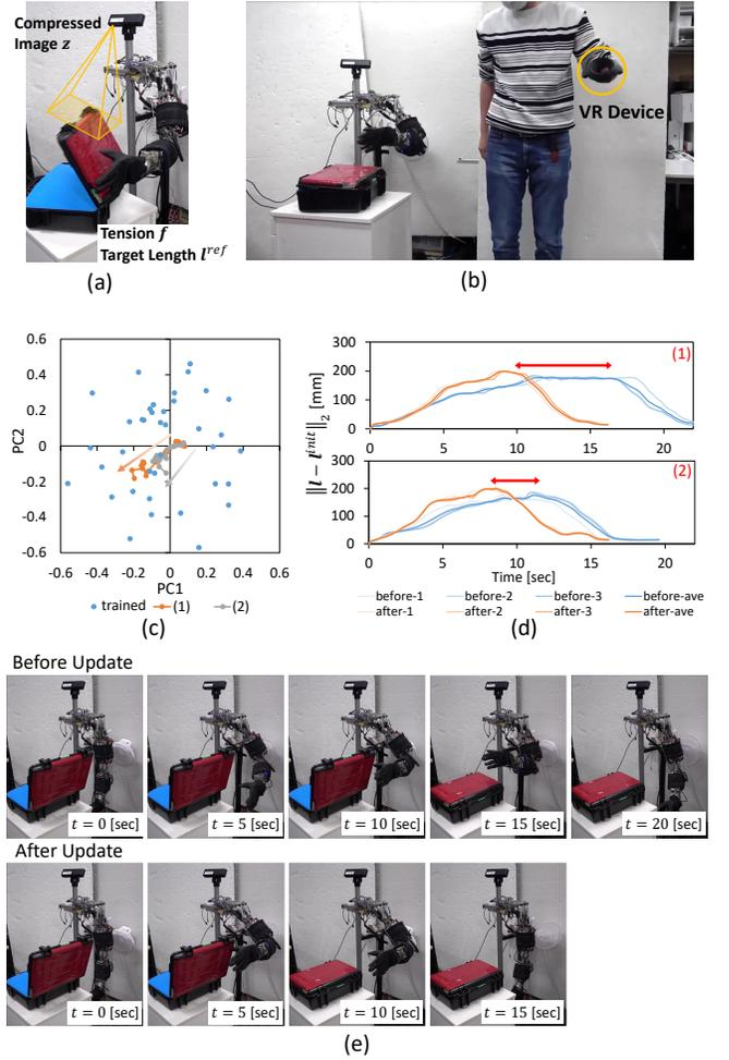
Fig. 8. Experiment of imitation learning considering motion style [10]. (a) shows the sensors and actuators of the musculoskeletal humanoid MusashiLarm, (b) shows the data collection setting using VR device, (c) shows the trained parametric bias and its trajectory when conducting online update of PB, (d) shows the trajectory of  $\|l - l^{init}\|_2$  when maximizing or not maximizing the muscle length velocity, and (e) shows the imitated motion of closing a box before and after the update of PB.
