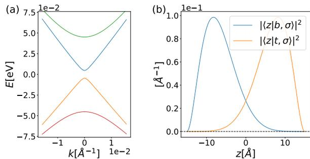
FIG. 3. (a) Energy spectrum of the translation-invariant MTI slab model in the QAH regime for thickness  $d = 30 \text{ \AA}$ ,  $\lambda = 25 \text{ meV}$  and  $\mu = 0$ . (b) Probability distributions  $|\langle z|l, \sigma\rangle|^2$ , where  $l \in \{t, b\}$ , associated with the top and bottom surface states of the slab for a thickness  $d = 30 \text{ \AA}$ .
