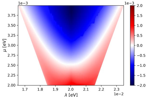
FIG. 14. Gap value  $\tilde{M}_1$  [see Eq. (12)] for an MTI/SC slab with thickness  $d = 30 \text{ \AA}$  and width  $W = 5200 \text{ \AA}$ . The parameters of the 2D model,  $m_0$ ,  $m_1$ , and  $v_F$  are taken from Table I and  $D = -1\text{eV\AA}^2$ , and we considered  $\Delta_1 = 2 \text{ meV}$ ,  $\Delta_2 = 0$ . The values we consider for  $\lambda$  and  $\mu$  correspond to the region with topological phase  $N = 1$  in the infinite 2D geometry.
