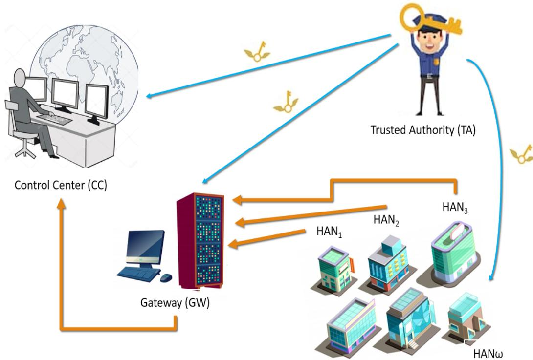
FIGURE 2.3: A typical model of the SG network
