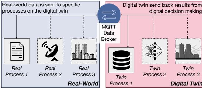
Fig. 5: An overview depicting how the MQTT communication broker facilitates bidirectional data distribution to specific processes, enabling scalable implementation of digital twins.
