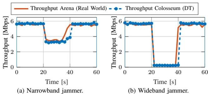
Fig. 8: Throughput results from jamming experiments on the Arena and Colosseum testbeds, showcasing narrowband and wideband cases, adapted from [7].
