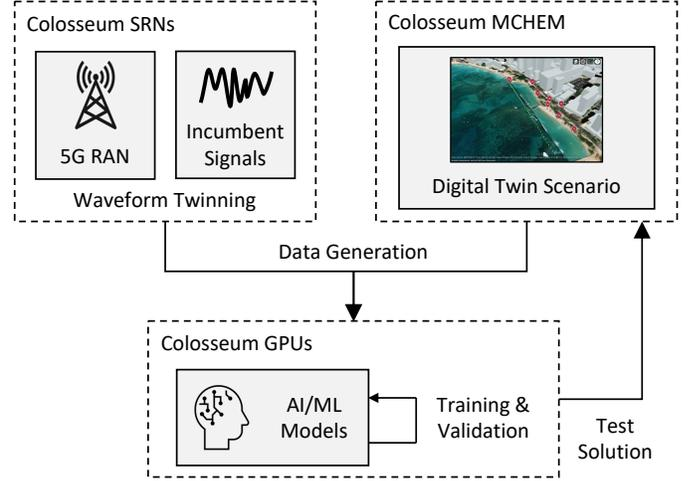
Fig. 7: Colosseum workflow for data-driven spectrum-sharing solutions development and testing.
