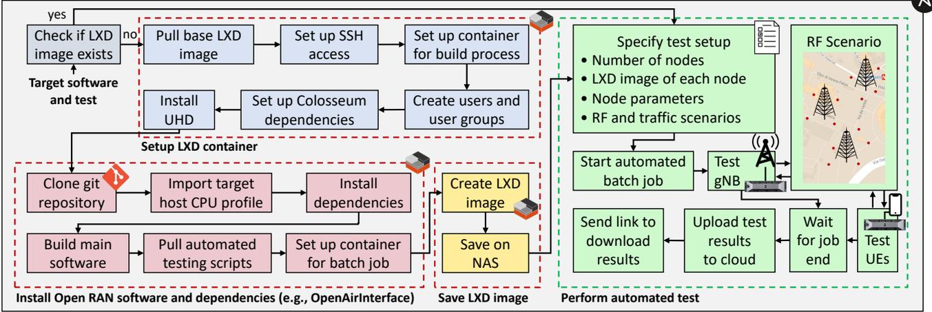
Fig. 4: Ansible pipeline to perform an automated test on Colosseum.
