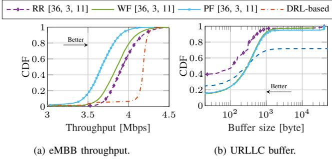
Fig. 6: Performance of a DRL agent controlling slicing and scheduling policies, from [15]. We compare the data-driven xApp and baselines without DRL-based adaptation. For the latter, the performance is based on the slicing configuration chosen with the highest probability by the best-performing DRL agent, and the three scheduler policies.
