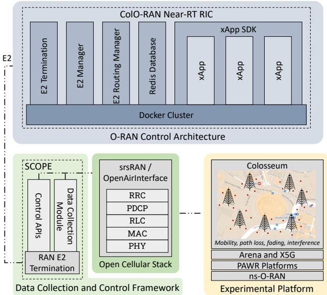
Fig. 2: Intelligent Control Loops with Colosseum, based on the OpenRAN Gym framework [19].
