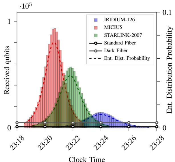
Fig. 3: Received qubits for various satellites overhead and fiber connections between Munich and Nuremberg with an average frame inter-arrival time of 20 ms between frames.
