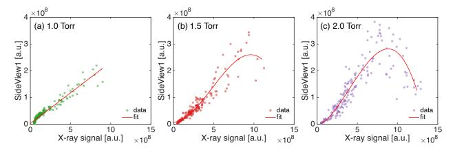
Fig. 6. Correlation between plasma light and x-ray signal. The plasma light detected by the sideview1 camera is plotted as a function of the x-ray signal for three datasets acquired at different pressures. The red lines are polynomial fits [with order one (linear) for (a) and three (cubic) for (b) and (c)] to illustrate the trend of the data.
