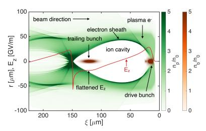
Fig. 1. Schematic of two-bunch plasma wakefield acceleration. An intense beam (drive bunch) ionizes lithium vapor to create plasma (illustrated by the green colormap) and excites a wake, characterized by an ion cavity enclosed by a plasma electron sheath. The red line indicates the
