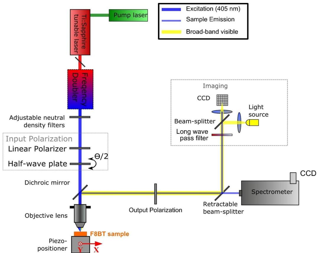
**Fig. S1** Experimental setup for the polarised  $\mu$ -PL spectral mapping measurements.
