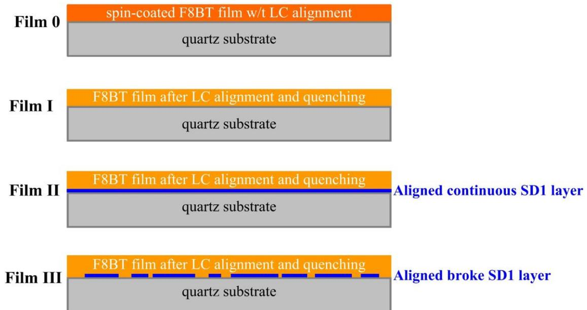
**Fig. S2** Illustration of the layer structure of the four kinds of F8BT films.
