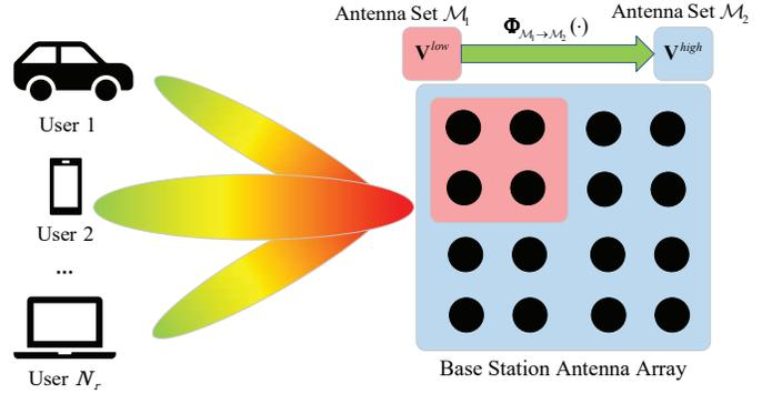
Fig. 1. The diagram shows the common system model. The function  $\Phi_{\mathcal{M}_1 \rightarrow \mathcal{M}_2}(\cdot)$  transforms the low-dimensional beamforming matrix from the antenna set  $\mathcal{M}_1$  to the high-dimensional beamforming matrix at  $\mathcal{M}_2$ .
