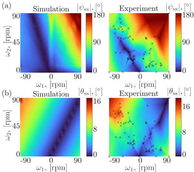
Fig. 6. The steady-state values of (a) yaw angle  $|\psi_{ss}|$  and (b) pitch angle  $|\theta_{ss}|$  are depicted in response to actuation speeds  $\omega_1$  and  $\omega_2$ . The generated maps represent results from simulations (left) and experiments (right), based on 180 and 75 trials, respectively.  $\times$  marks the experimental data points.
