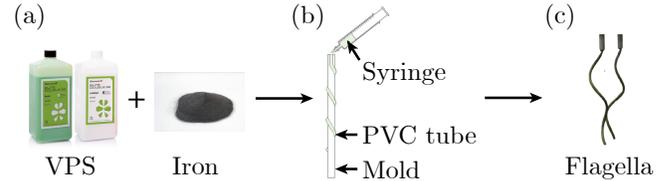
Fig. 3. Fabrication of a soft flagellum. (a) Step 1: blending VPS with iron powder to precisely calibrate the density of the silicone composite. (b) Step 2: using a syringe to inject the mixture into the PVC tube preformed by a mold. (c) Step 3: slitting the tube to extract the silicone elastomer.
