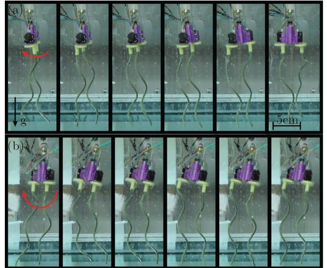
Fig. 1. Attitude adjustment of bi-flagellated robot in the viscous fluid (glycerin). (a) Rotation in the horizontal plane (pointing opposite to gravity direction). (b) Rotation in the vertical plane (pointing out to the paper).
