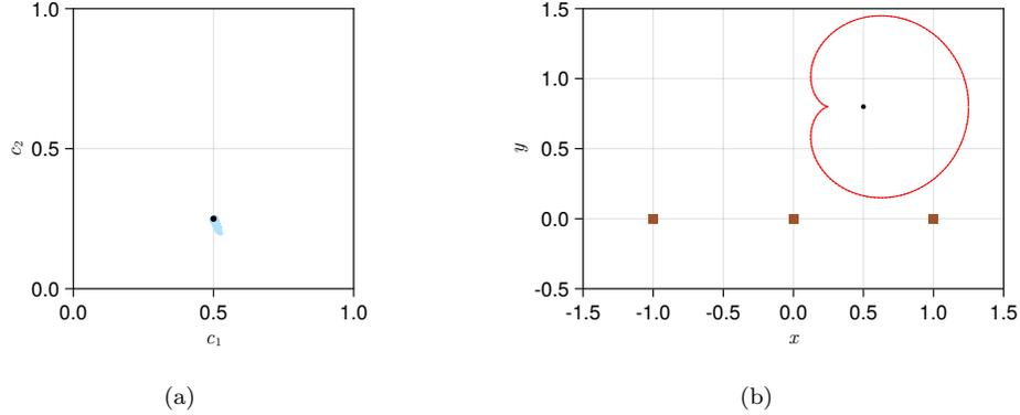
Figure 10: One true heater and one heater estimator with three temperature measurements. The position and strength of the heater are known and its shape is inferred. (a) samples on  $c_1 - c_2$  plot and (b) the red curve illustrates the boundary of the heater, with the solid line representing the true shape and the dashed line indicating the estimated shape. The black circles illustrate the true state.
