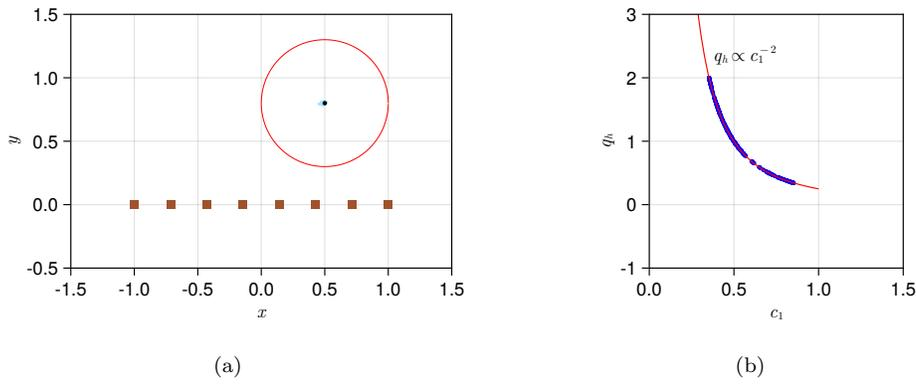
Figure 2: One true heater and one heater estimator with eight temperature sensors. The heater is given to be circular with radius  $c_1$  and true state  $(0.5, 0.8, 1, 0.5, 0)$ ; (a) samples generated with MCMC with the red curve representing the boundary of the heater, and (b) generated samples on  $q_h - c_1$  plot.
