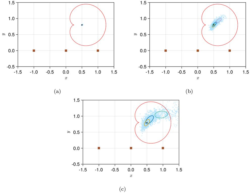
Figure 8: One true heater and one heater estimator with three temperature measurements, characterized by five Gaussian components for sensor noise equals to (a)  $5 \times 10^{-4}$ , (b)  $5 \times 10^{-3}$ , and (c)  $1 \times 10^{-2}$ . The red curve illustrates the boundary of the heater.
