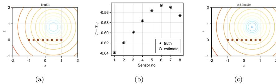
Figure 3: One true heater and one heater estimator with eight temperature measurements characterized by five Gaussian components. The heater is given to be a circle with radius  $c_1$  and true states  $(0.5, 0.8, 1, 0.5, 0)$ . (a) true temperature contours, (b) temperature distribution at the sensor locations, and (c) estimated temperature contours.
