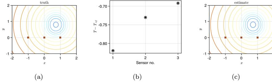
Figure 5: One true heater and one heater estimator with three temperature measurements characterized by five Gaussian components. The true state is given as  $(0.5, 0.8, 1, 0.5, 0.25)$  with *a priori* known shape. (a) true temperature contours, (b) temperature distribution at the sensor locations, and (c) estimated temperature contours.
