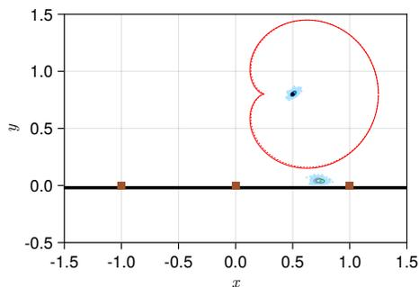
Figure 15: One true heater and one heater estimator with three temperature measurements, characterized by five Gaussian components for sensor noise equals to  $5 \times 10^{-3}$ . Sensors are placed on a wall with an adiabatic boundary condition. The red curve illustrates the boundary of the heater.
