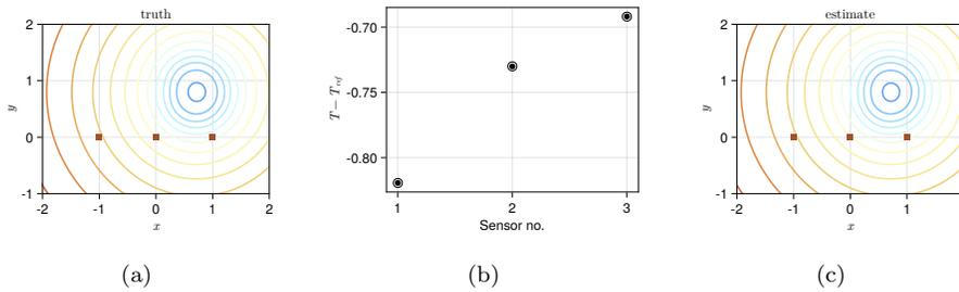
Figure 9: One true heater and one heater estimator with three temperature measurements. The position and strength of the heater are known and its shape is inferred. The true state is  $(0.5, 0.8, 1, 0.5, 0.25)$ .
