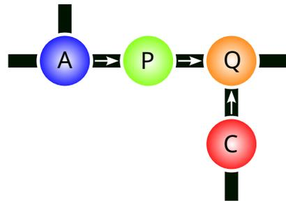
FIG. 6. The actual topology of qubits used in the test on *ibm\_brisbane* for the circuit in Fig. 3. The black connections indicate two-qubit gates linking the test qubits and external ones. The arrows show the direction of *ECR* gates between the test qubits (see Appendix B).
