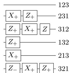
FIG. 4. The gate  $G_y$  for each permutation
