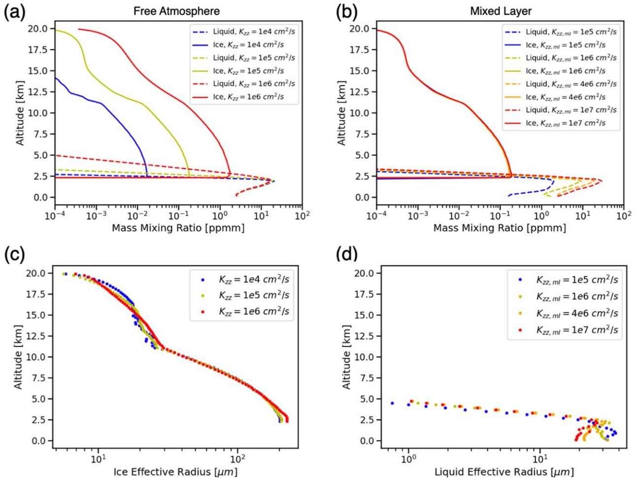
**Figure 8.** The effect of varying the diffusion coefficient. (a) and (b) Vertical distribution of ice (solid line) and liquid (dashed line) cloud mass mixing ratio when  $K_{zz}$  is varied in the free atmosphere (a) and the mixed layer (b). (c) Vertical distribution of ice particle effective radius when  $K_{zz}$  is varied in the free atmosphere. (d) Vertical distribution of liquid droplet effective radius when  $K_{zz}$  is varied in the mixed layer.
