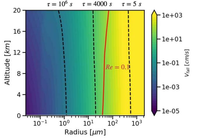
**Figure 1.** Terminal velocity of liquid droplets as a function of particle size and altitude for terrestrial conditions of gravity, temperature, and air composition. The red solid line indicates a Reynolds Number of 0.1. The black dashed lines indicate the time to fall through one of our 200 m-thick vertical levels:  $\tau = 5$  s,  $\tau = 4000$  s, and  $\tau = 10^6$  s.
