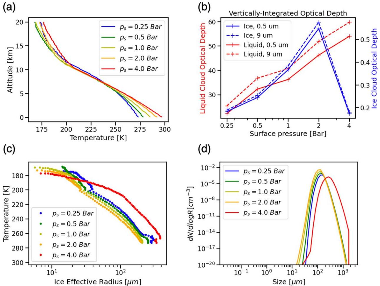
**Figure 9.** Effect of varying surface pressure on the following variables. (a) Temperature profile. (b) The ice (blue) and liquid (red) cloud optical depth at  $0.5 \mu\text{m}$  (solid line) and  $9 \mu\text{m}$  (dashed line) as a function of surface relative humidity. (c) Effective radius for ice clouds, and (d) distribution of ice cloud sizes at 7.5 km.
