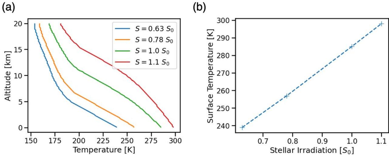
**Figure 2.** Thermal profiles from Clima, which are inputs for the CARMA simulations. (a) Temperature profiles with different stellar flux with all other parameters in Table 1 at the base case values. The green line for  $S = 1.0 S_0$  is the input for the default experiment. (b) The dependence of surface temperature with stellar flux. The surface temperature is a monotonic function of the stellar flux.
