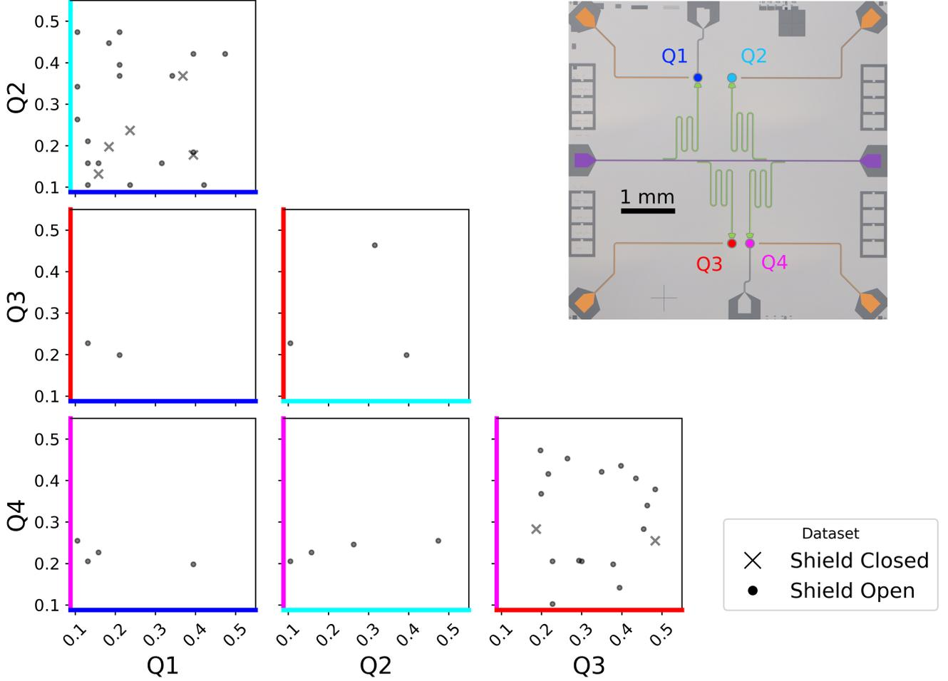
Figure 2: Correlated jump magnitudes  $0.1e \leq |\Delta q| \leq 0.5e$  for all qubit pairs, for SC (x's) and SO (dots), in units of electric charge,  $e$ . The raw data retains sign information, but only magnitude  $|\Delta q|$  is presented here for visual clarity. Non-correlated events are omitted, also for visual clarity. (Inset) A micrograph of the qubit chip, annotated with false colors to match the plot axes.
