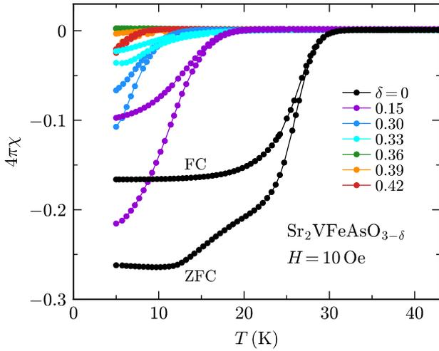
**Fig. 2.** (Color online) Temperature dependence of magnetic susceptibility of  $\text{Sr}_2\text{VFeAsO}_{3-\delta}$  in zero-field-cooling (ZFC) and field-cooling (FC) conditions under  $H = 10$  Oe.
