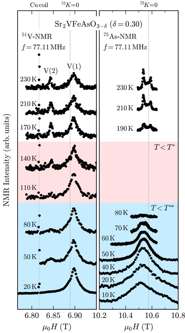
**Fig. 7.** (Color online)  $^{51}\text{V}$ - and  $^{75}\text{As}$ -NMR spectra in  $\text{Sr}_2\text{VFeAsO}_{3-\delta}$  with  $\delta = 0.30$  for various temperatures. The vertical dashed lines display the resonance fields corresponding to zero Knight shift ( $^{51/75}K = 0$ ). The signal from a Cu coil is indicated by the vertical dotted line.
