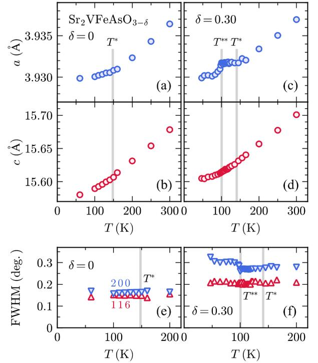
**Fig. 6.** (Color online) Temperature dependence of (a)  $a$ - and (b)  $c$ -axis lattice parameter of  $\text{Sr}_2\text{VFeAsO}_{3-\delta}$  for  $\delta = 0$ . (c), (d) Same as (a), (b) but for  $\delta = 0.30$ . The data were taken on the warming process.  $T^*$  and  $T^{**}$ , determined from  $\chi(T)$ , are indicated by the vertical gray lines. Temperature dependence of the full width at half maximum (FWHM) of the 200 and 116 peaks for (e)  $\delta = 0$  and (f)  $0.30$ .
