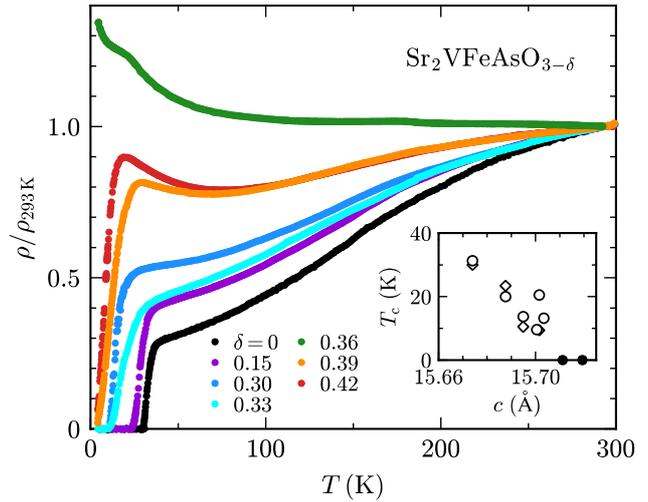
**Fig. 3.** (Color online) Temperature dependence of resistivity  $\rho$  of  $\text{Sr}_2\text{VFeAsO}_{3-\delta}$  normalized at 293 K. Inset shows the variation of  $T_c$  as a function of the  $c$ -axis lattice parameter. The  $T_c$  values were determined from the onset of magnetic susceptibility (open circles) and zero resistivity (open diamonds). The samples for which superconductivity was not observed in this study are indicated by closed circles.
