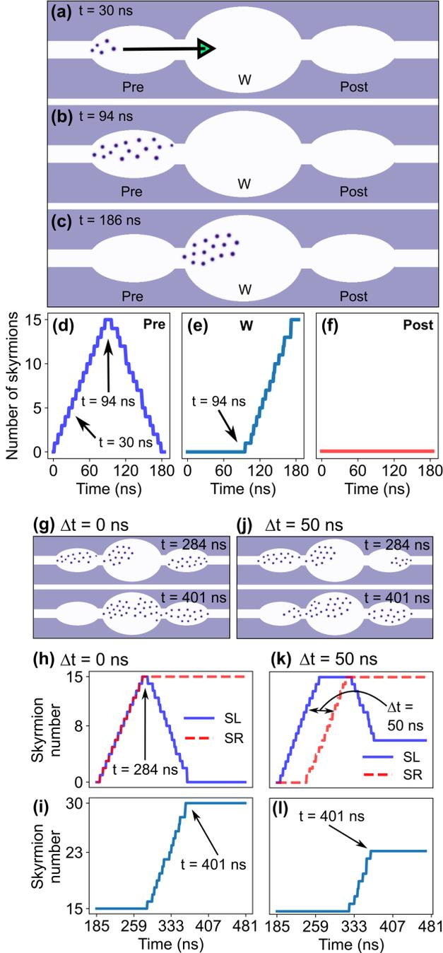
FIG. 3. Initial weight operation and comparative analysis of  $\Delta t = 0$  and  $\Delta t = 50$  ns spikes for LTP. (a-c) Magnetization simulation
