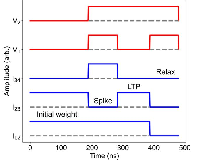
FIG. 2. Sequence and timing of currents ( $I_{12}$ ,  $I_{23}$ ,  $I_{34}$ ), voltages ( $V_1$ ,  $V_2$ ), and key operations (initial weight, spike on the left/right, LTP, system relaxation) in the skyrmion chamber device during the long-term potentiation process.
