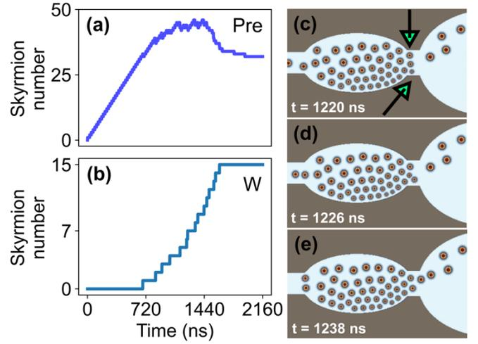
FIG. 5. Natural motion of skyrmions to mimic plasticity. (a) The weight at Pre shows the 32 skyrmion threshold for leakage to (b)  $W$  and (c) shows a magnetization snapshot for skyrmions moving from Pre to  $W$  at  $t = 1220$  ns, (d)  $t = 1226$  ns and (e)  $t = 1238$  ns. Arrows show the forces applied to a skyrmion. Color represents  $M_z$  from  $-1$  (red) to  $+1$  (blue).
