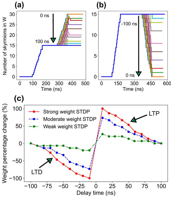
FIG. 4. STDP plasticity behavior and dendritic location-based plasticity rates. (a) LTP STDP: Skyrmion count in  $W$  over time for  $\Delta t = 0-100$  ns. (b) LTD STDP: Skyrmion count in  $W$  for  $\Delta t = -100$  to 0 ns. (c) Dendritic location-based STDP plasticity rates - strong (0-100% weight change), moderate (7-73%), weak (0-27% LTP, 0-20% LTD).
