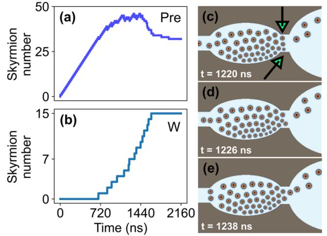
FIG. 5. Natural motion of skyrmions to mimic plasticity. (a) The weight at Pre shows the 32 skyrmion threshold for leakage to (b)  $W$  and (c) shows a magnetization snapshot for skyrmions moving from Pre to  $W$  at  $t = 1220$  ns, (d)  $t = 1226$  ns and (e)  $t = 1238$  ns. Arrows show the forces applied to a skyrmion. Color represents  $M_z$  from  $-1$  (red) to  $+1$  (blue).
