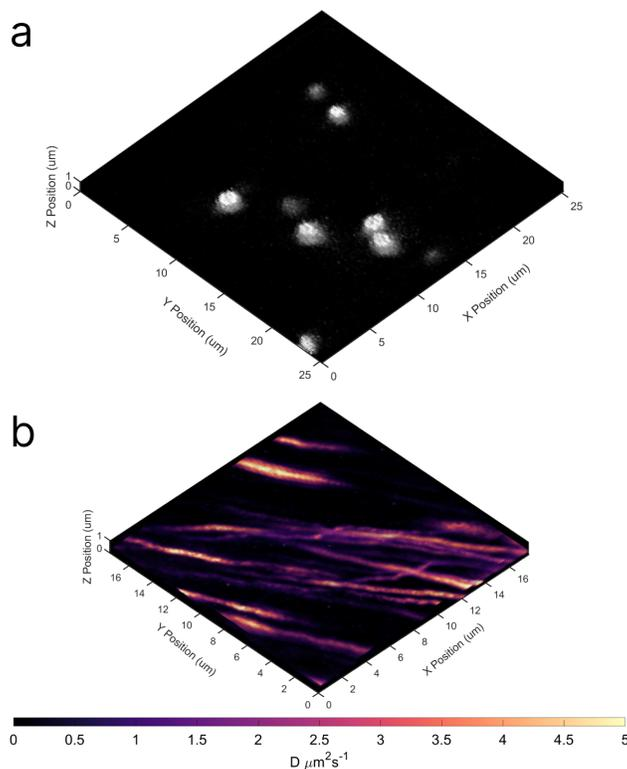
FIG. 9. 3D reconstruction of stationary  $2 \mu\text{m}$  beads (a) and dynamic 155 kDa dextran (b) in a 2 wt% agarose gel generated using our 3D reconstruction code from data collected on our home-built LSM.
