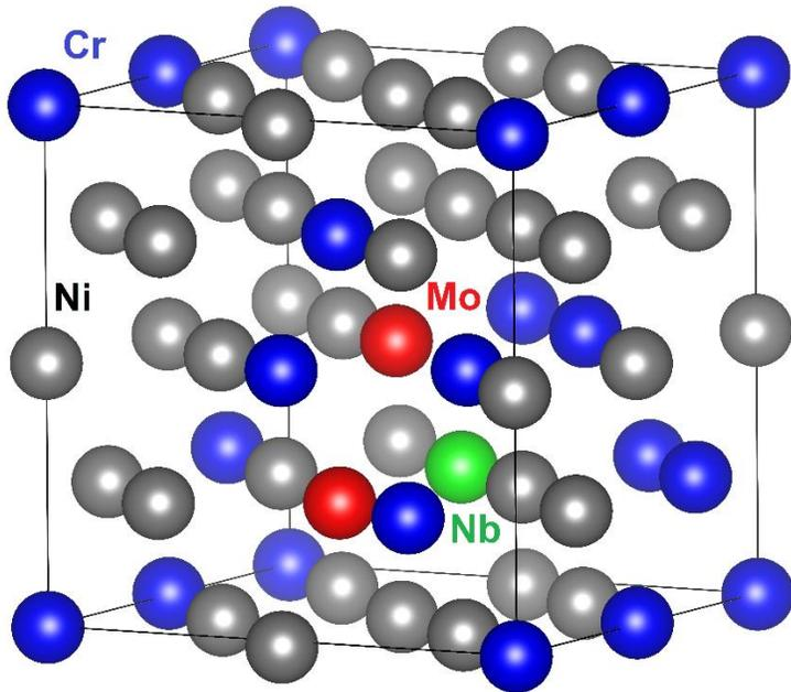
Figure S 1. One of the 32-atom supercells for IN625 (i.e., the configuration SCRAP<sub>f</sub>) based on the composition of Ni<sub>21</sub>Cr<sub>8</sub>Mo<sub>2</sub>Nb<sub>1</sub>.
