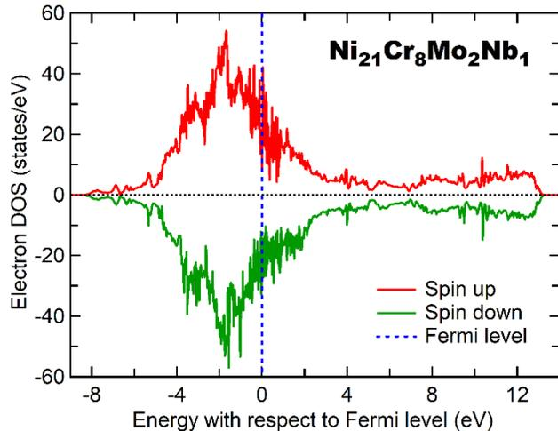
Figure S 4. Electronic density of states of  $\text{Ni}_{21}\text{Cr}_8\text{Mo}_2\text{Nb}_1$  at the equilibrium volume of  $\text{SCRAP}_f$ .
