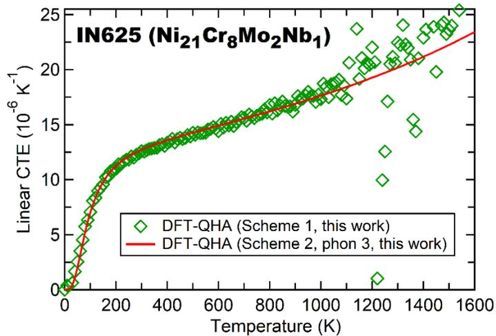
Figure S 6. Predicted values of linear CTE of IN625 by DFT-based QHA using Scheme 1 (Sch. 1) and Scheme 2 (Sch. 2, with  $F_{vib}$  fitted by 3 parameters using Eq. (2) at each  $T$ , labeled as phon 3), respectively, see also Figure 3b for more CTE results.
