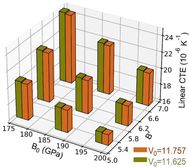
Figure 4. Sensitivity of the predicted linear CTE of IN625 at 1500 K with respect to the changes of equilibrium properties at 0 K with data in Table S 2, i.e.,  $B_0$  ( $187.7 \pm 10.9$  GPa),  $B'$  ( $5.95 \pm 0.78$ ), and  $V_0$  ( $11.691 \pm 0.066 \text{ \AA}^3/\text{atom}$ ).
