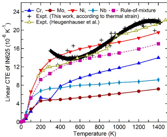
Figure S 2. Experimental linear CTE values of pure elements as recommended by Touloukian et al. [17]. The results of IN625 are based on the present measurements and those by Heugenhauser et al. [18]. The predicted CTE values of FCC-based Ni<sub>21</sub>Cr<sub>8</sub>Mo<sub>2</sub>Nb<sub>1</sub> are based on the rule-of-mixture of CTE values of pure elements (in this figure).
