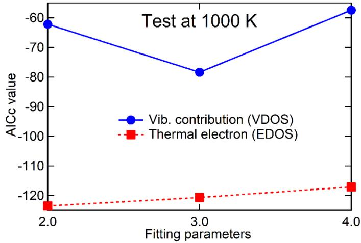
Figure S 5. Predicted AICc values regarding vibrational contribution  $F_{vib}(V, T)$  via phonon DOS's and thermal electronic contribution  $F_{el}(V, T)$  via electronic DOS's to free energy at 1000 K; see Figure 2.
