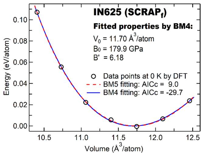
Figure 1. Data points at 0 K by DFT-based final static calculations for the configuration  $\text{SCRAP}_f$ , together with the fitted  $E$ - $V$  EOS curves using 4 parameters (BM4) and 5 parameters (BM5) of Eq. 2. The fitted properties (see Table S 2) and the calculated AICc values are also listed on this plot.
