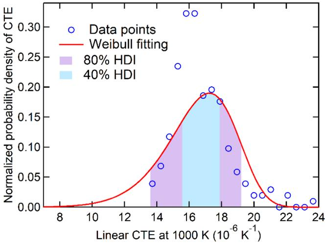
Figure S 8. Distribution of the predicted CTE values of IN625 at 1000 K according to 200 predictions using the selected 200 datasets in Figure S 7. The red line shows the fitting of Weibull distribution, and two areas show the percentages of *highest density interval* (HDI) according to the Weibull distribution.
