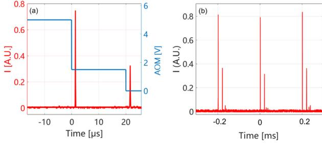
**Fig. 4.** Experimental results on the generation of two sub-pulses sequence. (a) The double-step driving signal on the AOM (blue curve) and the corresponding dual laser pulses. (b) Zoom-out of the dual-pulse train.
