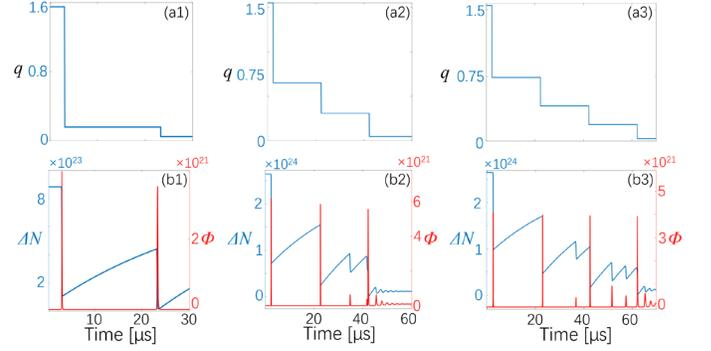
**Fig. 1.** Numerical simulation of the sub-pulse generation via multi-step Q-switching. (a1-a3): the step-like variation of intracavity Loss  $q$  with different steps from 2 to 4; (b1-b3): the corresponding results of population inversion (blue line) and sub-pulse sequence (red line), respectively.
