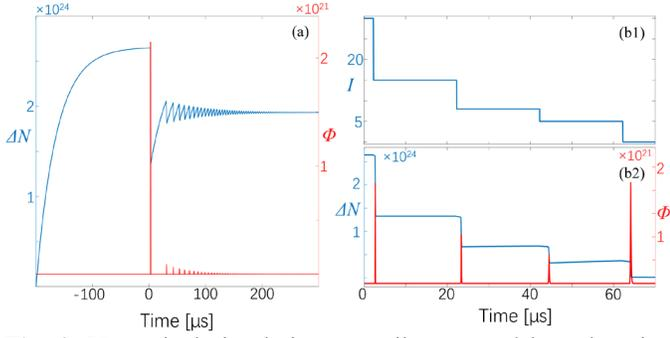
**Fig. 2.** Numerical simulation on spikes caused by relaxation oscillation in different pump intensity (a): The following spikes after a giant Q-switching pulse generation while the pump intensity is a constant. (b): Inhibition of the spikes in four sub-pulses via modulation of the pumping,  $I_{pump}$  refers to the pump intensity.
