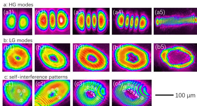
**Fig. 7.** Beam profiles of the sub-pulses with  $HG_{(n,0)}$  modes patterns and their convert results. (a) original HG modes direct generated from Q-switching resonator, from  $HG_{(1,0)}$  to  $HG_{(30,0)}$ , respectively; (b) LG modes converted from the HG modes above, respectively; (c) self-interference patterns, showing the topological charge of each LG modes.
