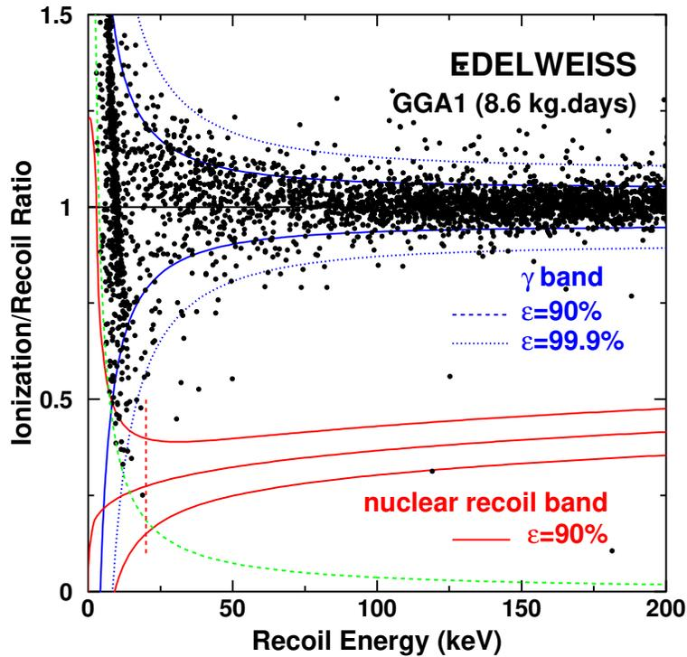
Figure 2. Scatter diagram of the ionisation efficiency, normalized to electron recoils, as a function of recoil energy for all events with energy  $< 200$  keV recorded by the EDELWEISS experiment in the fiducial volume of a 320 gram Ge detector (from Ref.). With an effective mass 600 smaller than the DAMA NaI crystals, and an exposure 10 000 times shorter, this detector exceeds by a factor  $> 5$  the sensitivity of the DAMA experiment.
