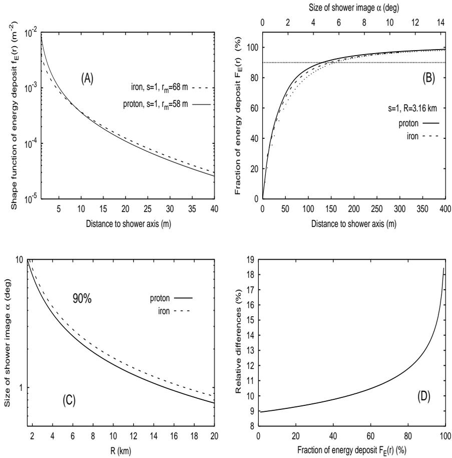
Fig. 10. (A) Shape of energy deposit density  $f_E(r)$  for vertical 10 EeV proton and iron showers. (B) Integral of energy deposit versus distance to shower axis for proton shower (solid line) and iron (dashed line). (C) Size of shower in age containing 90% of fluorescence light versus detector to shower distance  $R$ . (D) Relative difference in the shower in age between iron and proton shower.
