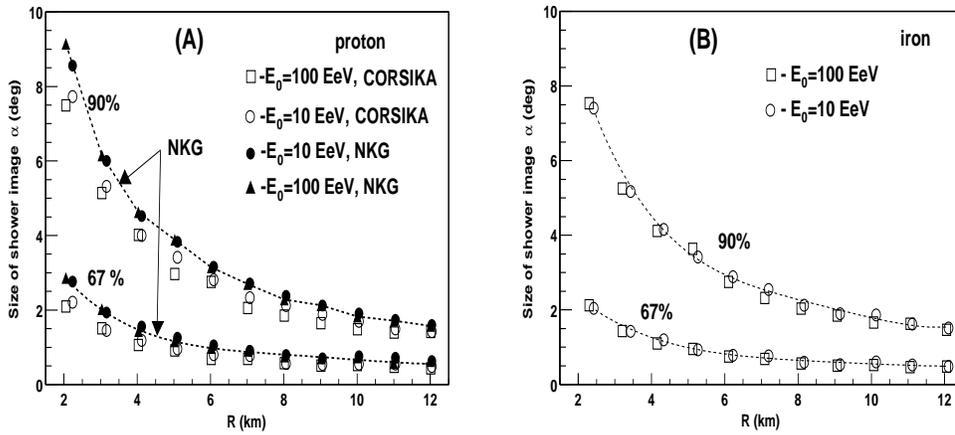
Fig. 12. (A) Size of the shower image at shower maximum containing 90% and 67% of light versus the detector to shower distance  $R$ , using the CORSIKA and NKG distributions of energy deposit. The dashed line corresponds to shower image obtained with constant value of fluorescence yield  $n_0 = 4.02 \text{ photons/m}$ . (B) Size of the shower image containing 90% and 67% of light versus  $R$  using the CORSIKA distributions of energy deposit for iron (showers at different energies).
