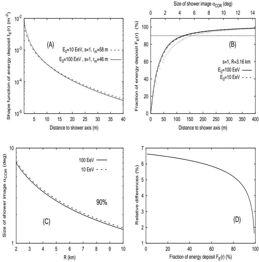
Fig. 7. (A) Shape of energy deposit density  $f_E(r)$  for vertical proton showers with energies 100 EeV and 10 EeV derived from CORSIKA. (B) Integral of energy deposits versus distance to shower axis. (C) Size of shower image containing 90% of fluorescence light versus detector-to-shower distance  $R$ . (D) Relative difference in the shower image size between proton showers with energies 10 EeV and 100 EeV.
