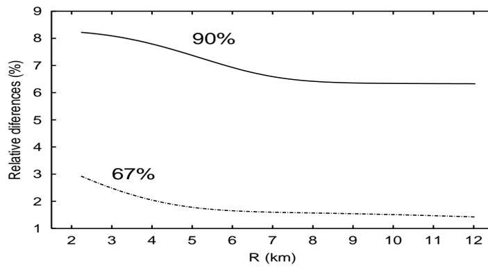
Fig. 4. Relative difference between size of shower in age calculated using total light and only fluorescence versus the detector-to-shower (R) distance for a vertical shower with energy 10 EeV .
