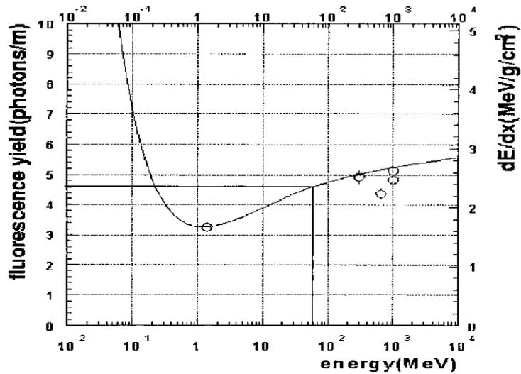
Fig. 1. Energy dependence of nitrogen fluorescence between 300 and 400 nm in dry air at the pressure 760 mm Hg. The scale of fluorescence yield is adjusted so that the 1.4 MeV point lies on the  $dE/dX$  curve (taken from Ref. [11]).
