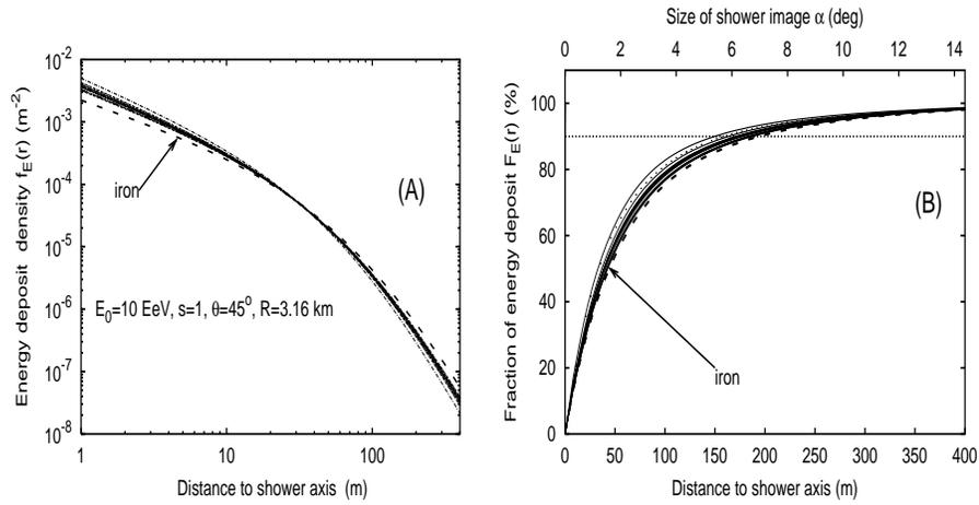
Fig. 11. (A) Lateral distribution of energy deposit calculated for 15 single proton showers (solid lines) and average of 5 iron showers (dashed lines) at energy  $E_0 = 10 \text{ EeV}$ . (B) Integral of the energy deposits versus distance to shower axis for proton showers (solid lines) and iron ones (dashed line).
