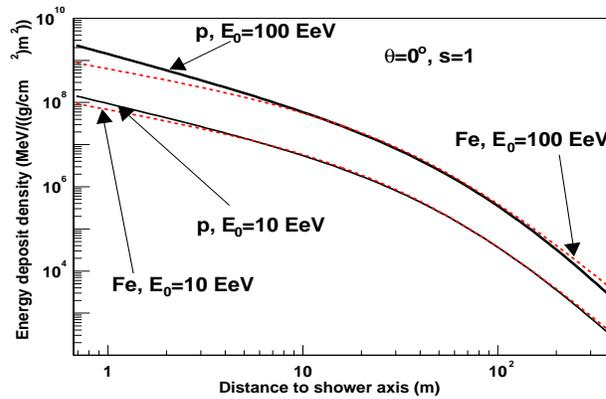
Fig. 9. Comparison of the average lateral distributions of energy deposit density calculated for an average iron and proton showers with different energy.
