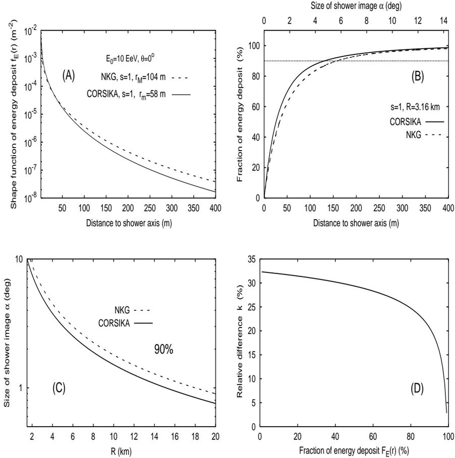
Fig. 6. (A) Shape of particles density  $f_E(r)$  in the CORSIKA and NKG approximations. (B) Integral  $F_E(r)$  of shape functions  $f_E(r)$  from Figure 6A. (C) Size of shower image containing 90% of fluorescence light versus the detector-to-shower distance  $R$ . (D) Relative difference between shower image size obtained in the CORSIKA and NKG approaches, see text for more details. Vertical showers at energy 10 EeV are presented.
