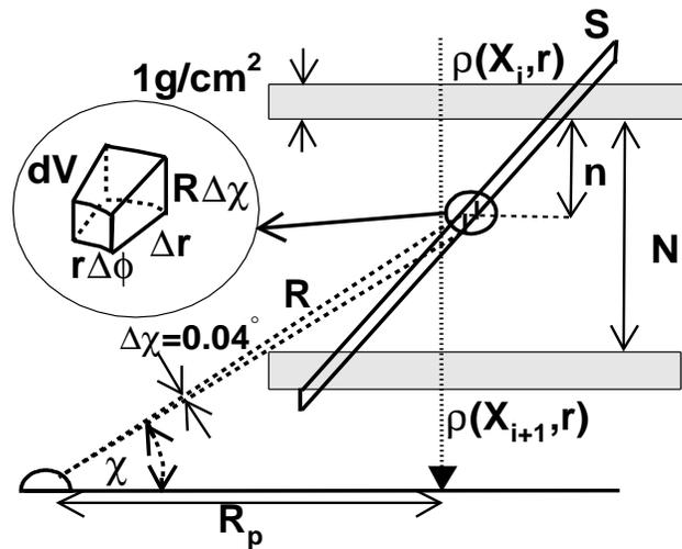
Fig. 2. Geometry of an EAS as seen by the fluorescence detector. Photons which arrive simultaneously to the FD originate from surface S. See text for more details.
