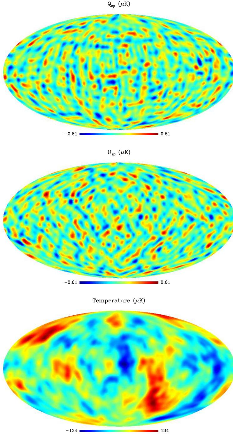
**Fig. 6.** Contamination maps for  $Q$  (top) and  $U$  (mid) generated by the convolution between the  $\Pi$  beam of the SPOrt horn and the Temperature map of a  $\Lambda$ CDM model (concordance model as from WMAP first year results). The Temperature map, smeared by the FWHM  $\sim 7^\circ$  beam, is also shown (bottom).
