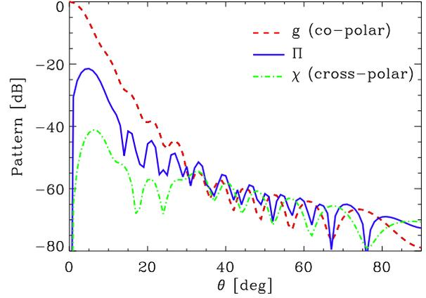
**Fig. 3.** Amplitude of the instrumental polarization pattern  $\Pi$  for the 90 GHz feed horn of the SPOrt experiment along a radial cut. The pattern is normalized to the maximum of the main beam. The co-polar and the cross-polar beams along the  $45^\circ$  cut are also shown for comparison.
