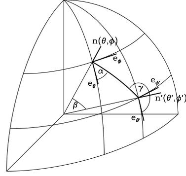
**Fig. 5.** The position of  $\hat{\mathbf{n}} = (\theta, \phi)$  with respect to  $\hat{\mathbf{n}}' = (\theta', \phi')$  is defined by three angles:  $\beta$ , the angular separation between the two versors;  $\alpha$ , the angle to take  $\hat{\mathbf{e}}_\theta(\hat{\mathbf{n}})$  in right-handed sense onto the great circle connecting  $\hat{\mathbf{n}}$  and  $\hat{\mathbf{n}}'$ ;  $\gamma$ , the same as  $\alpha$  but referred to  $\hat{\mathbf{e}}_\theta(\hat{\mathbf{n}}')$ .
