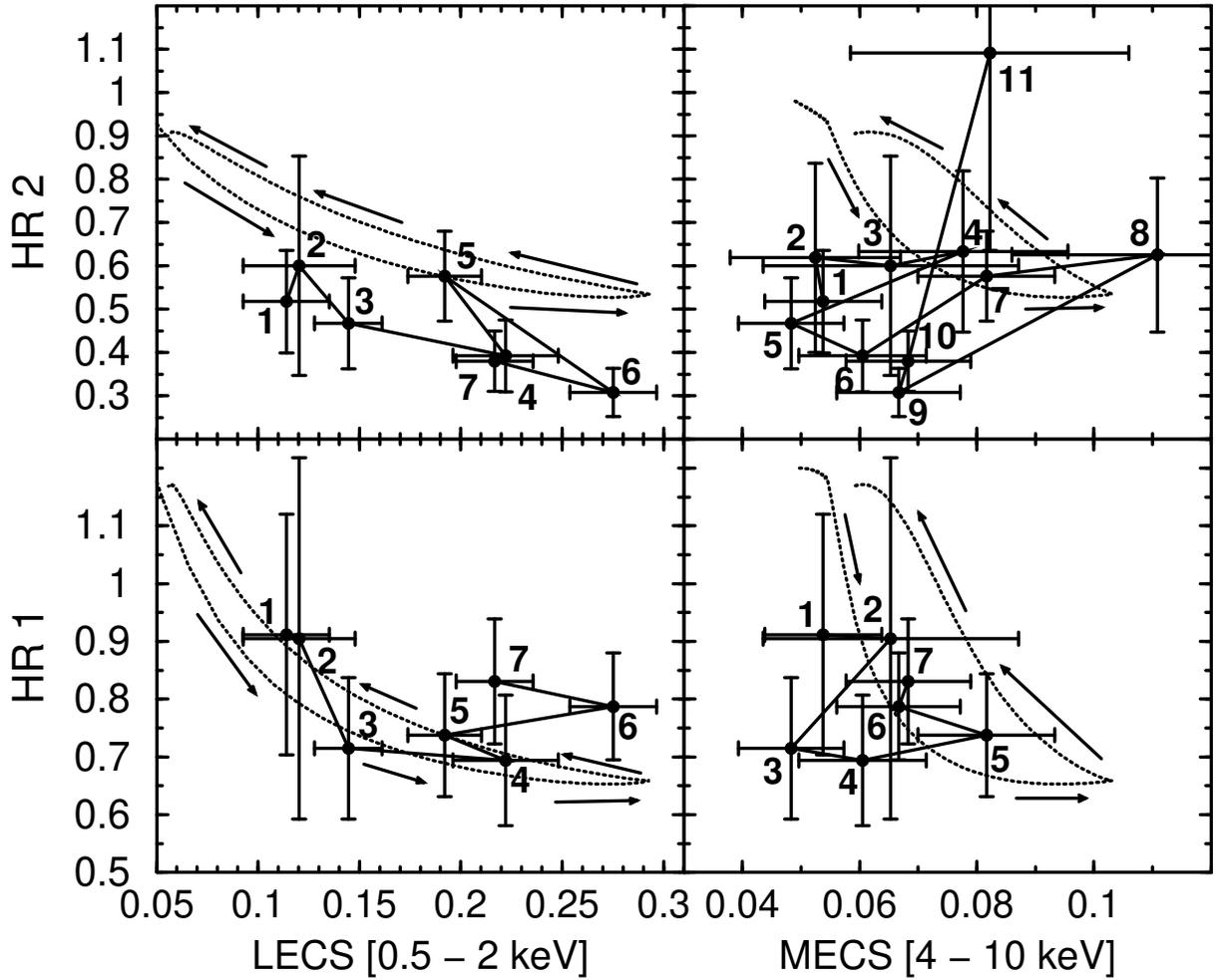
Fig. 12. Hardness-intensity diagram of the BeppoSAX hardness ratios HR1 and HR2 as defined in  $x2$  vs. soft X-ray LECS and medium-energy MECS flux for the well-resolved X-ray source at  $t = 0.5$  (6.5 h) of Nov. 1, 2000 (data from Ravasio et al. 2003). The dotted curves indicate the simulated spectral hysteresis curves from our best-fitting scenario (Fig. 10).
