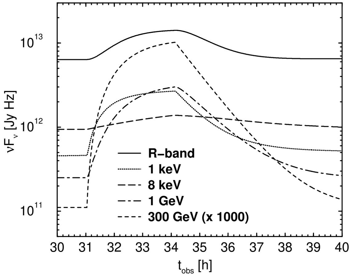
Fig. 11. Model light curves from the  $t$  illustrated in Fig. 10. The 300 GeV light curve has been shifted up by a factor of  $10^3$  in order to  $t$  on the same scale as the other light curves.
