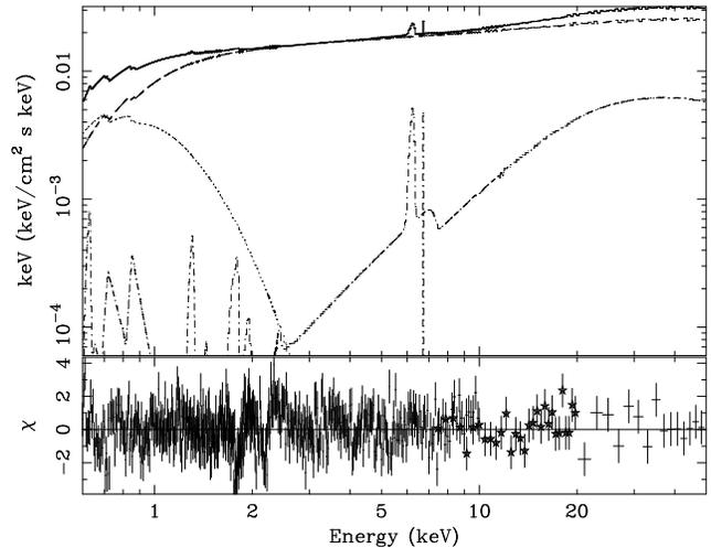
**Figure 6.** The upper panel shows a broadband model of 3C 120 using two 1xFeIONDISC models and a bremsstrahlung continuum. The solid line plots the total model, while the individual curves denote the model components. The bottom panel plots the residuals (in units of standard deviations). PCA data are denoted by stars.
