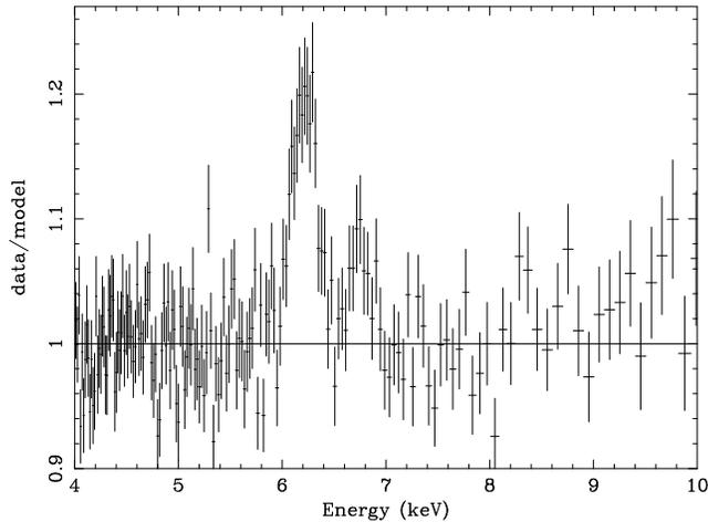
**Figure 3.** The data-to-model ratio between 4 and 10 keV, for an absorbed power-law fit to the 3–50 keV data. The data between 5 and 7.2 keV were ignored in the fit to emphasize the emission features in the iron line region.
