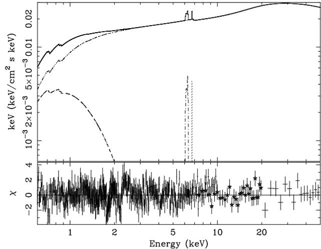
**Figure 5.** The upper panel shows the best-fitting broadband model of 3C 120 using a PEXRAV and bremsstrahlung continuum, plus edges from O VII and O VIII. The solid line plots the total model, while the individual curves denote the model components. The bottom panel plots the residuals (in units of standard deviations). PCA data are denoted by stars.
