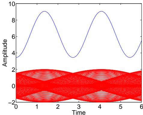
Figure 1: Plot illustrating the nonstationarity of a randomly shifted waveform that has been undersampled and then reconstructed. The upper curve is the sixth moment<sup>7</sup>. The lower curve shows the process envelope. The original process is given by Equation 3 with  $\alpha = 1.0$ ,  $\beta = 3.0$ ,  $\theta \in [0, 1)$ , and  $\Delta t = e$ .
