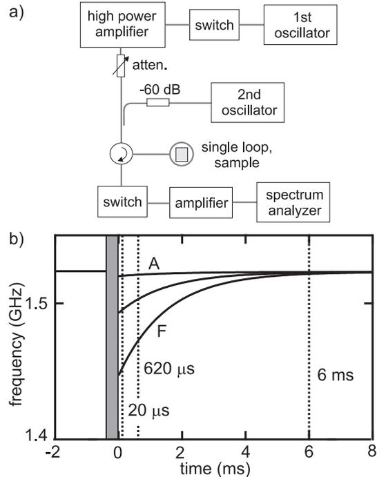
FIG. 1. (a) Schematic experimental setup. Details are given in the text. (b) Experimental measurement road map. The horizontal line for  $t < 0$  identifies the AFMR frequency. During the high power driving pulse (shaded area) the detection electronic is blocked. The solid lines A ... F show the AFMR for increasing pump-pulse power levels. The vertical dotted lines identify different time-cuts described in the text.
