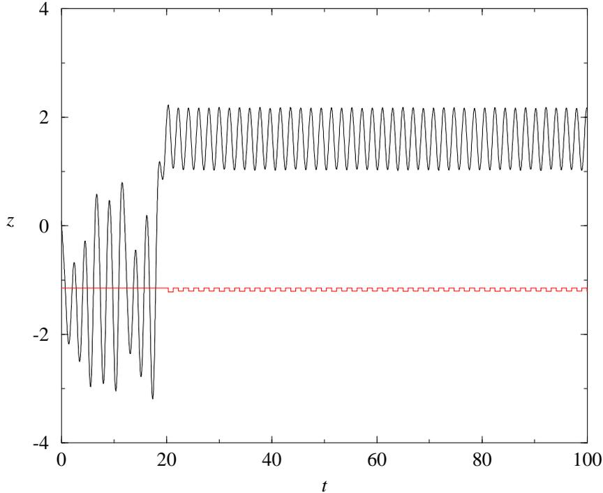
Figure 4: The fuzzy controller stabilizes a previously unstable period-1 orbit. The control is switched on at time 20. The lower trace shows the correction pulses applied by the controller.
