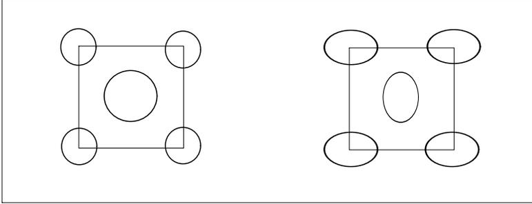
FIG. 1. Minimum unit cells for the two dot architectures considered in this paper with two different circular dots (left) and two identical, but rotated, ellipsoidal dots (right).
