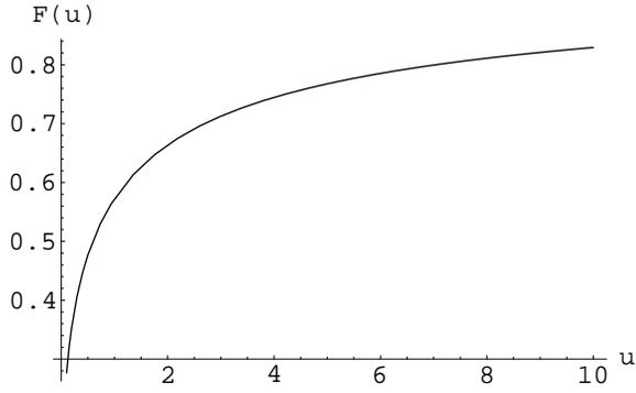
Fig 4. The scaling function  $\mathcal{F}(u)$  describes the growth of load fluctuations with depth for the 1+1 dimensional  $q$ -model close to the critical point [see eqs (7) and (50)]. Injection is neglected.
