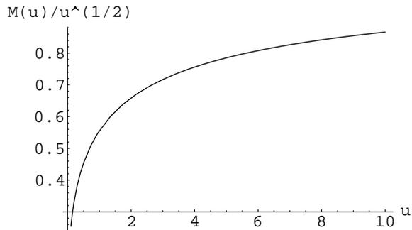
Fig 5. Growth of load fluctuations with depth for the 1+1 dimensional  $q$ -model close to the critical point. The scaling function  $\mathcal{M}(u)$  gives the contribution due to fluctuations in the weight of beads [eqs (79) and (102)]. Here  $\mathcal{M}(u)/\sqrt{u}$  is plotted as a function of  $u$ .
