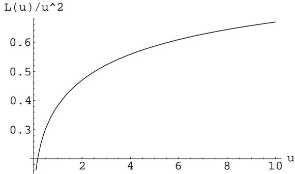
Fig 7. Growth of load fluctuations with depth for the 1+1 dimensional  $q$ -model close to the critical point. The scaling function  $\mathcal{L}(u)$  gives a contribution proportional to the square of the average weight of beads [eqs (79) and (102)]. Here  $\mathcal{L}(u)/u^2$  is plotted as a function of  $u$ .
