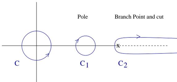
Fig 10. Contours for inverting the  $z$  transform.
