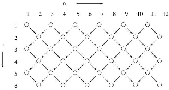
Fig 1. The  $q$ -model of stress propagation through a bead pack in 1+1 dimensions. The beads are assumed to sit on a regular lattice. Each bead is supported by its two nearest neighbours in the layer below.
