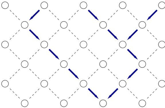
Fig 2. *Scheidegger's model*: For the singular  $q$ -model the load zig-zags down lines that merge but do not split. In Scheidegger's model of river basins these lines are interpreted as tributaries merging to form a river.
