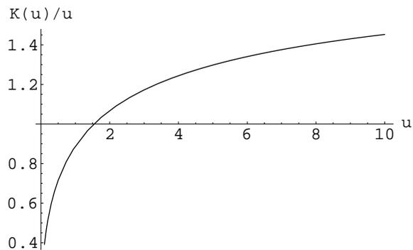
Fig 6. Growth of load fluctuations with depth for the 1+1 dimensional  $q$ -model close to the critical point. The scaling function  $\mathcal{K}(u)$  gives a contribution proportional to the average weight of beads [eqs (79) and (102)]. Here  $\mathcal{K}(u)/u$  is plotted as a function of  $u$ .
