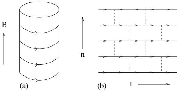
Fig 3. A *quantum Hall multilayer*: Layers of two dimensional electron gases are stacked vertically and a strong perpendicular magnetic field is applied. The important electronic states are at the edge of each layer. These chiral edge states propagate in the direction shown in (a). A quantum network model for the surface of the multilayer is shown in (b).
