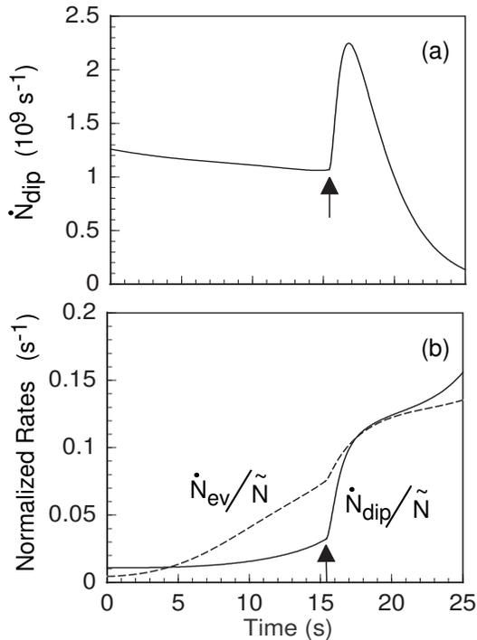
FIG. 3. Time evolution of (a) the dipolar loss rate  $\dot{N}_{\text{dip}}$ , and (b) normalized rates,  $\dot{N}_{\text{ev}}/\tilde{N}$  (dashed line) and  $\dot{N}_{\text{dip}}/\tilde{N}$  (solid line). The dipolar loss rate exceeds the evaporation rate at around 17.5 s. The arrow indicates the point at which the BEC transition occurs.
