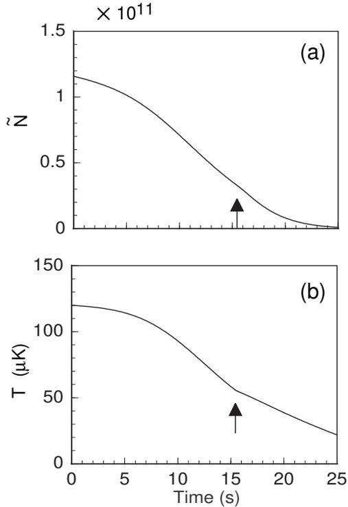
FIG. 1. Time evolution of (a) the total number of trapped atoms  $N$ , and (b) temperature  $T$ . The arrow indicates the point at which the BEC transition occurs. The heating due to the dipolar spin relaxation occurs after the BEC transition.
