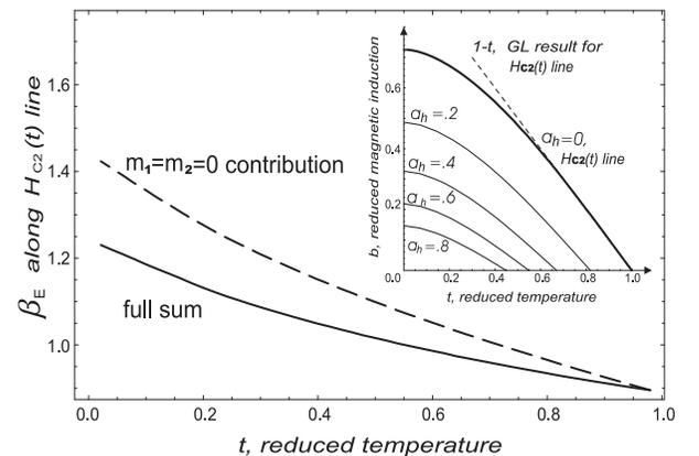
FIG. 1. Energy parameter  $\beta_E$  for the hexagonal lattice along  $H_{c2}(t)$  line presented as a function of temperature: dashed line — the contribution of the first term in Eq. (20) with  $m_1 = m_2 = 0$ , solid line — the full sum. Insert: Contour plot of the parameter  $a_h$  as a function of  $t$  and  $b$ . Magnetic induction is normalized to produce  $db/dt = -1$  at  $t = 1$ .
