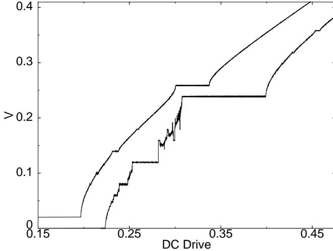
FIG. 1. Velocity  $V$  vs applied DC drive  $f_{DC}$  for AC amplitudes  $A = 0.25$  (upper curve) and  $0.35$  (lower curve) for a square pinning array. The upper curve has been offset upwards by  $0.02$  for clarity.
