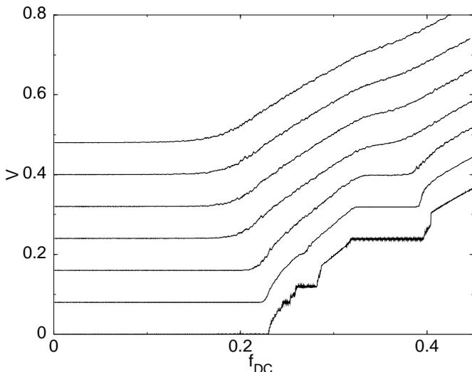
FIG. 10. The  $V$  vs  $f_{DC}$  curves for different temperatures for  $B/B_\phi = 2.0$  and  $A = 0.35$ . The curves have been shifted up from zero for presentation. From lowest to highest,  $T/T_m = 0.0, 0.07, 0.28, 0.64, 0.75, 0.87,$  and  $0.96$ , where  $T_m$  is the melting temperature.
