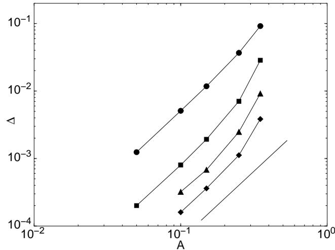
FIG. 7. The scaling of the step width  $\Delta$  as a function of AC amplitude  $A$  for the fractional steps corresponding to: (diamonds)  $f_{DC} = 0.235$  [Fig. 3(a)], (triangles)  $f_{DC} = 0.243$  [Fig. 3(b)], and (squares)  $f_{DC} = 0.28$  [Fig. 3(c)]. The scaling of the main step at  $f_{DC} = 0.36$  [Fig. 3(e)] is also shown (circles). The solid line is a quadratic fit.
