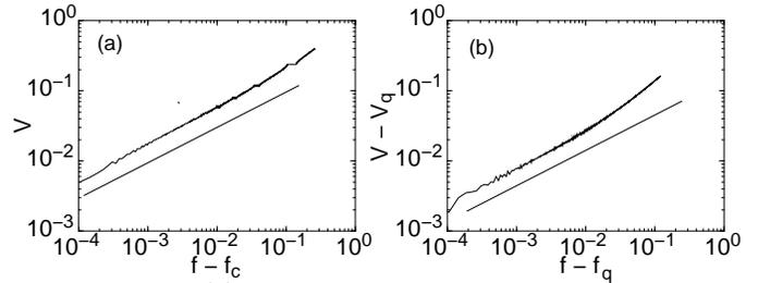
FIG. 5. (a) Log-log plot just above depinning of  $V = (f - f_c)$  for  $A = 0.35$ , where  $f_c = 0.196$  is the depinning threshold and  $f$  is the DC driving force. The solid line shows a slope of  $\beta = 1/2$ . (b) Log-log plot above the main step of  $V - V_q = (f - f_q)$  where  $V_q = 0.24$  is the velocity along the main step and  $f_q = 0.395$  is the DC driving force where the step ends. The solid line shows a slope of  $\beta = 1/2$ .
