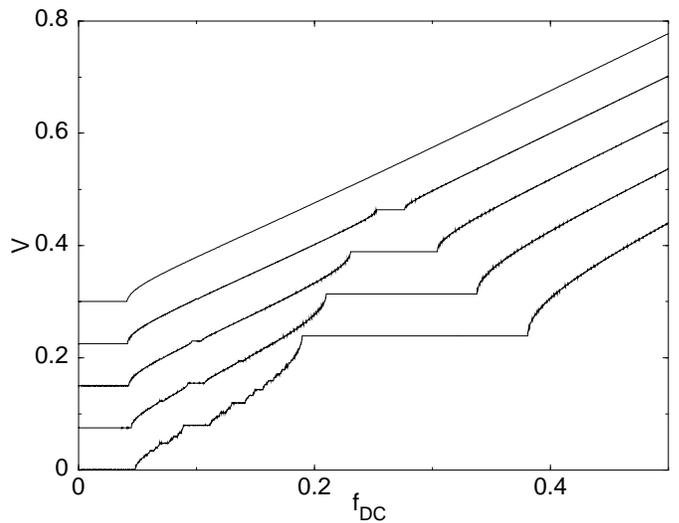
FIG. 11. The velocity  $V$  vs DC driving force  $f_{DC}$  curves for a triangular pinning array at different AC amplitudes  $A$ . The system size and pinning density are the same as for the system in Fig. 1. The curves have been shifted up for presentation. From lowest to highest,  $A = 0.35, 0.25, 0.15, 0.05,$  and  $0.0$ .
