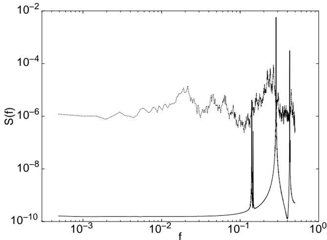
FIG. 4. Velocity noise  $S(f)$  versus frequency  $f$  for  $A = 0.35$ . Lower curve: Noise signature along the main step corresponding to the vortex orbit at  $f_{DC} = 0.36$  shown in Fig. 3(e). Upper curve: Noise signature in the non-step region for the vortex orbit at  $f_{DC} = 0.305$  shown in Fig. 3(d).
