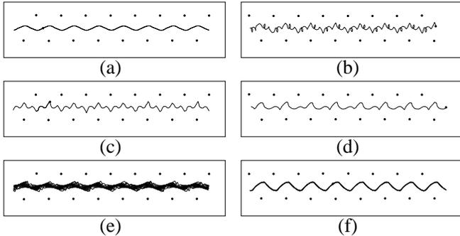
FIG. 12. Vortex trajectories for triangular pinning on various steps for (a)  $A = 0.0$  and (b-f)  $A = 0.25$ . (a) For  $A = 0.0$  above depinning,  $f_{DC} = 0.3$ , there is a periodic transverse motion of the vortex even for zero AC drive. Remaining panels:  $A = 0.25$  and (b)  $f_{DC} = 0.07$ , (c)  $f_{DC} = 0.11$ , (d)  $f_{DC} = 0.1375$ , (e)  $f_{DC} = 0.2$ , and (f)  $f_{DC} = 0.3$ .
