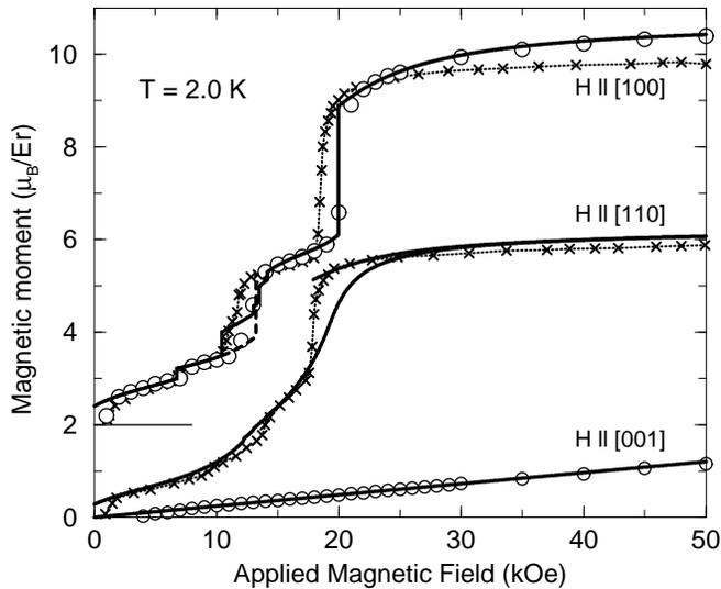
FIG. 2: The magnetization curves of  $\text{ErNi}_2\text{B}_2\text{C}$  at 2 K. The open circles are the experimental results of Cho *et al.*<sup>13</sup>. The crosses connected by dashed lines show the experimental results of Canfield *et al.*<sup>2</sup>. The remaining solid and dashed lines are the calculated results. The experimental and theoretical results in the case of  $H \parallel [100]$  have been shifted upwards by 2 units.
