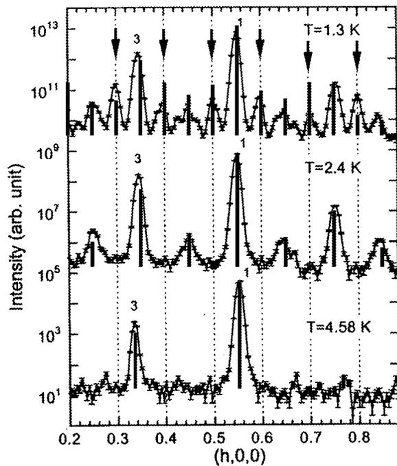
FIG. 3: Scan along  $[h, 0, 0]$  at  $T = 1.3$  K, 2.4 K, and 4.38 K, measured with unpolarized neutrons. The data have been offset for clarity. The figure is a copy of Fig. 1 from Ref. [4] in which the calculated diffraction patterns in the different cases (the heavy solid lines) have been incorporated.
