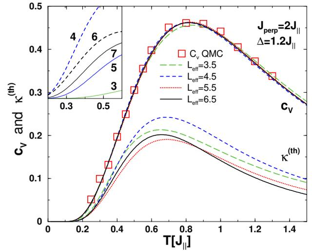
FIG. 2. Temperature dependence of  $\kappa^{(th)}$  and the dimensionless specific heat for ladders with twisted boundary conditions and  $J_{\perp} = 2J_{\parallel}$ . Both magnitudes are computed using the average procedure (5) described in the text. The specific heat for a 200-ladder computed with QMC is plotted for comparison (squares). Inset  $\kappa^{(th)}$  for  $L = 3, 5, 7$  (from bottom up) and  $L = 4, 6$  (from top down) in the low-temperature region.
