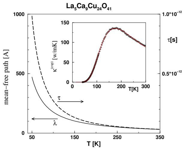
FIG. 4.  $\tau$  (right-scale) and  $\lambda$  (left-scale) for  $\text{Ca}_9\text{La}_5\text{Cu}_{24}\text{O}_{41}$  extracted using Eq. (6). The experimental data by Hess et al.<sup>7</sup> is shown in the inset (red circles) together with an analytic  $\tau$  (solid line) discussed in the text.
