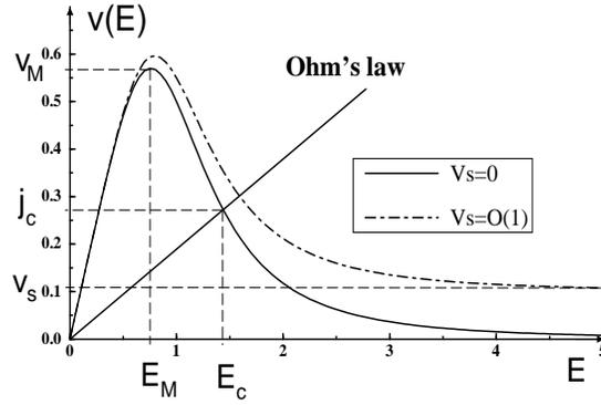
FIG. 1. Drift velocities and Ohm's law.  $v(E) = |\vec{v}(\vec{E})|$  has a maximum  $v_M = 3^{3/4}/4$  at  $E = E_M = 1/3^{1/4}$  (for  $v_s = 0$ ), followed by a region of negative differential mobility for  $E > E_M$ . At large fields  $E \gg 1$ , the electron velocity monotonically decreases to a value  $v_s$ , which may be zero.
