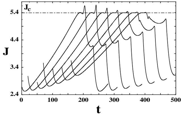
FIG. 5. Current vs time during one period of the self-oscillations for  $\phi \in (0.35, 0.5)$ . Values of  $\phi$  are: 0.36, 0.38, 0.4, 0.42, 0.44, 0.46 and 0.48, depicted from left to right, and the critical current at which a new wave is nucleated is  $J_c = 5.39$ .
