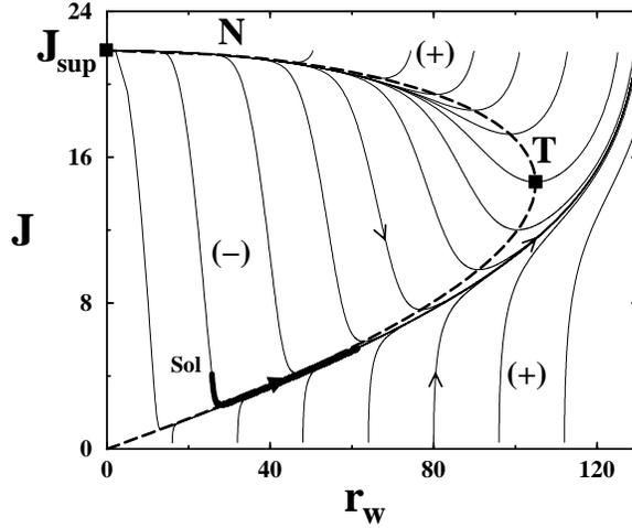
FIG. 13. Phase plane  $(r_w, J)$  showing the nullcline  $dJ/dr_w = 0$  (dash line) and the turning point for  $v_s = 0$  and a bias  $\phi = 0.6$ . The thick line represents the trajectory of the solution for initial data  $J(0) = 4.1$  and  $r_w = 26$ , until  $J_c \approx 5.4$  is reached.
