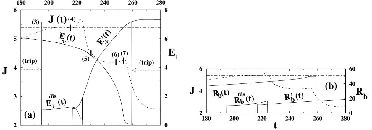
FIG. 7. Evolution of  $J(t)$  and  $E_+(t)$  during one oscillation period for  $\phi = 0.38$  and  $v_s = 0$ . (a) Stage in which there are multiple pulses. (b)  $R_b(t)$  during the multi-pulse stage.  $R_b^{dis}(t)$  and  $R_b'(t)$  are the locations of the maximum fields of the transient field disturbance and of the new pulse, respectively. Marked times are: (3) 195, (4) 215, (5) 230, (6) 248, and (7) 253.
