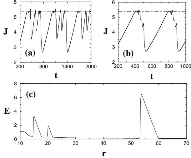
FIG. 10. (a) Complex current signal  $J(t)$  for  $\phi = 0.5$  and a time interval  $\Delta t \approx 650$ . (b) Same for  $\phi = 0.52$  and  $\Delta t \approx 400$ . (c) Three-pulse electric field profile for  $\phi = 0.52$  and  $\Delta t \approx 400$ . In all cases,  $v_s = 0$ . In (a) and (b), the horizontal line marks the critical current  $J_c$ .
