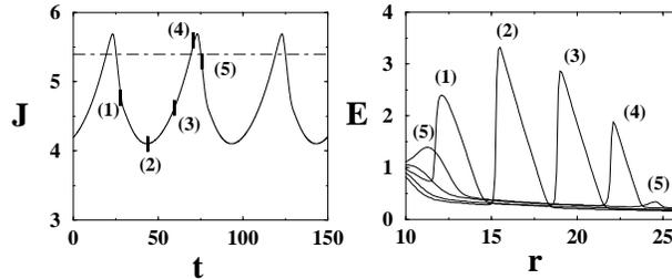
FIG. 3. Total current density (left) and electric field profiles (right) for  $\phi = 0.18$ . The electric field profiles are depicted at the times marked on the graph of  $J(t)$ . The horizontal line in the latter corresponds to the value  $J_c$ .
