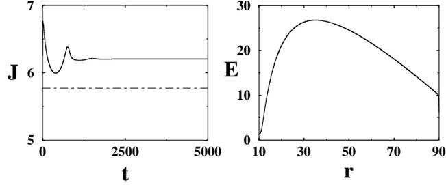
FIG. 4. Stationary solution for  $\phi = 20$ ,  $L = 80$  and  $v_s = 0.1$ .  $J$  evolves towards  $J \approx 6.2$  greater than  $J_c = 5.77$ . The maximum electric field,  $E_+ \approx 26.75$ , is reached at  $R_b \approx 35.12$ . Field values at the boundaries are  $E(r_c) = 1.25$  and  $E(r_a) = 0.14$ .
