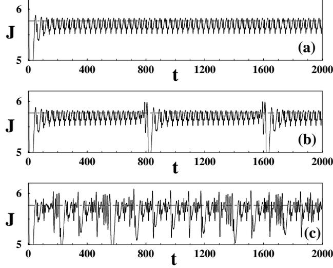
FIG. 12. Complex current signals for  $v_s = 0.1$ ,  $r_c = 10$ ,  $r_a = 50$  and several bias values: (a)  $\phi = 0.41$  (periodic signal), (b)  $\phi = 0.411$  (periodic signal with a longer period due to current bursts), and (c)  $\phi = 0.42$  (aperiodic signal). In all cases,  $J(t)$  oscillates about  $J_c = 5.77$  with an approximate amplitude of 0.5.
