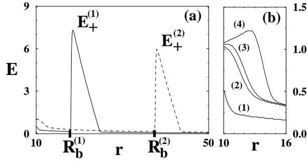
FIG. 8. (a) Electric field profile during the the single-pulse stage at times (1) and (2) of Fig. 6. (b) Details of the field profile near the cathode: the slope at  $r_c$  increases with  $J$ ;  $dE(r_c)/dr = 0$  for  $J = J_c \approx 5.24$  at time (3).
