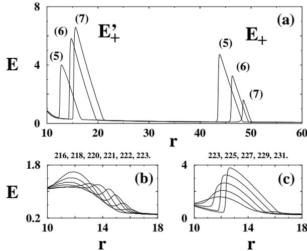
FIG. 9. (a) Electric field profiles during the multi-pulse stage at times marked as (5), (6) and (7) in Fig. 6 for  $\phi = 0.38$  and  $v_s = 0$ . (b) Details of the unsuccessful attempt at shedding one pulse from the cathode for  $J < J_c$ . (c) Successful nucleation of the new pulse after time (4).
