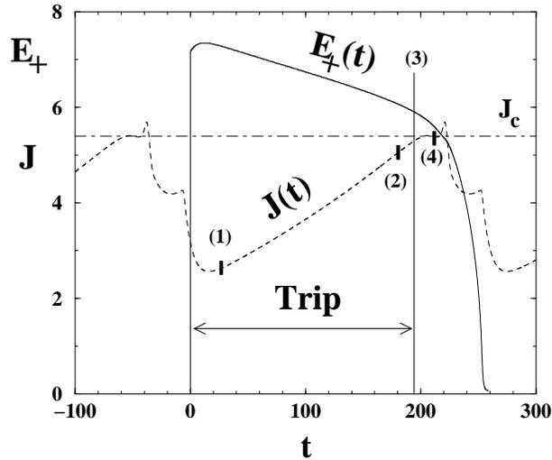
FIG. 6. Evolution of  $J(t)$  and  $E_+(t)$  during one oscillation period for  $\phi = 0.38$  and  $v_s = 0$ , during the time interval  $0 < t < \Delta t \approx 200$ , where there is a single pulse in the sample. Marked times are: (1) 30, (2) 180, (3) 195, (4) 215.
