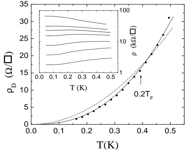
FIG. 1.  $\rho_D$  vs  $T$  for sample A. Layer densities are matched at  $p = 2.5 \times 10^{10} \text{ cm}^{-2}$ . Provided are the best  $T^2$  (dashed line) and  $T^{2.5}$  (solid line) fits. Inset:  $\rho$  vs  $T$  for the bottom layer. From top to bottom,  $p = 0.80, 0.85, 0.90, 1.0, 1.2, 1.4,$  and  $2.0 \times 10^{10} \text{ cm}^{-2}$ .
