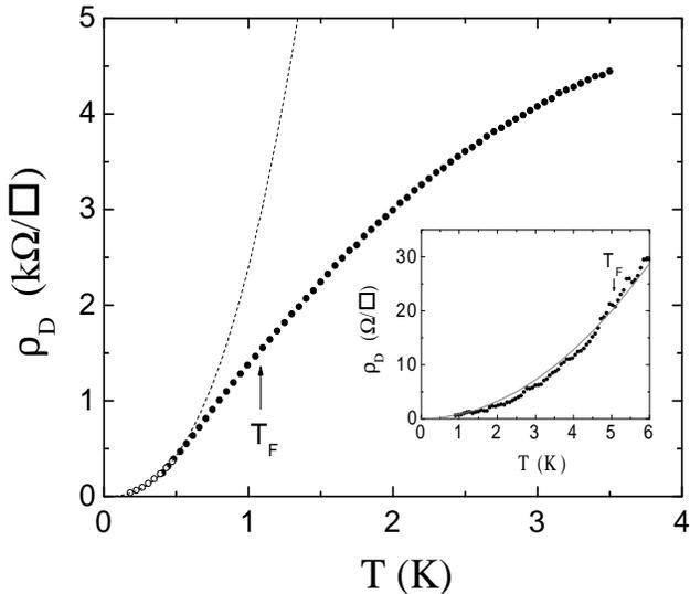
FIG. 2.  $\rho_D$  vs  $T$  for sample A. Layer densities are matched at  $p = 1.5 \times 10^{10} \text{ cm}^{-2}$ . Data measured in the dilution refrigerator are shown with open circles. Also shown is the best  $T^{2.5}$  fit of these points. Inset:  $\rho_D$  vs  $T$  for sample B, whose layer densities are matched at  $p = 7.0 \times 10^{10} \text{ cm}^{-2}$ . Also shown is the best  $T^2$  fit of the data. The Fermi temperature is indicated on both plots.
