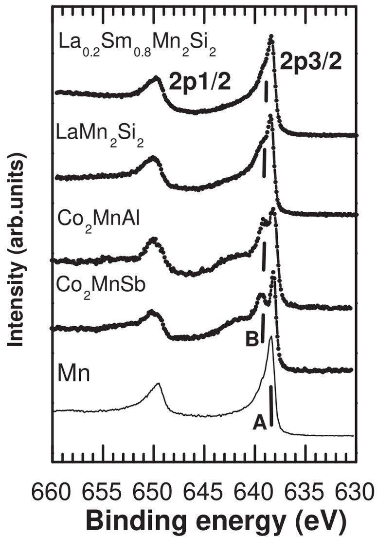
FIG. 2: Mn 2p X-ray photoemission spectra.
