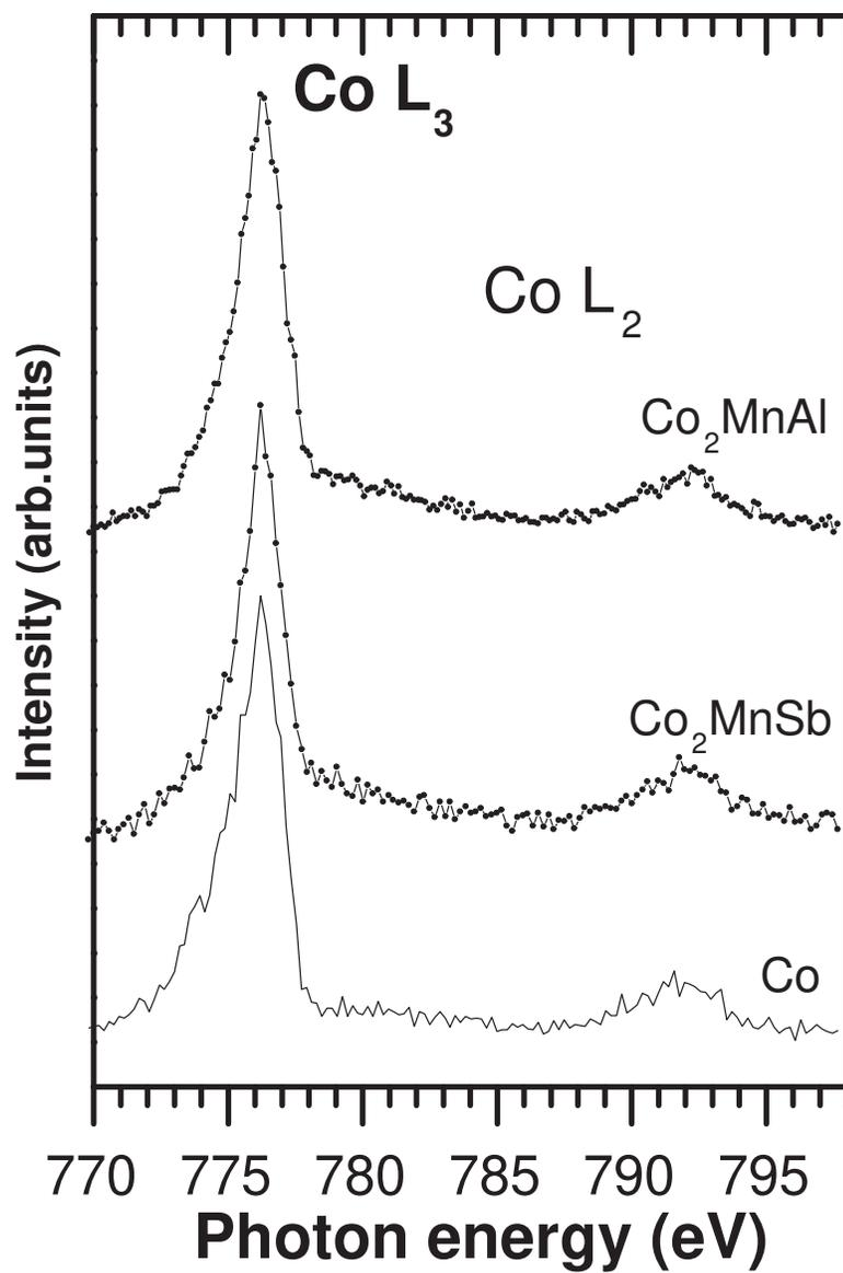
FIG . 6:  $\text{Co } L_{2,3}$  X-ray emission spectra of Heusler alloys.
