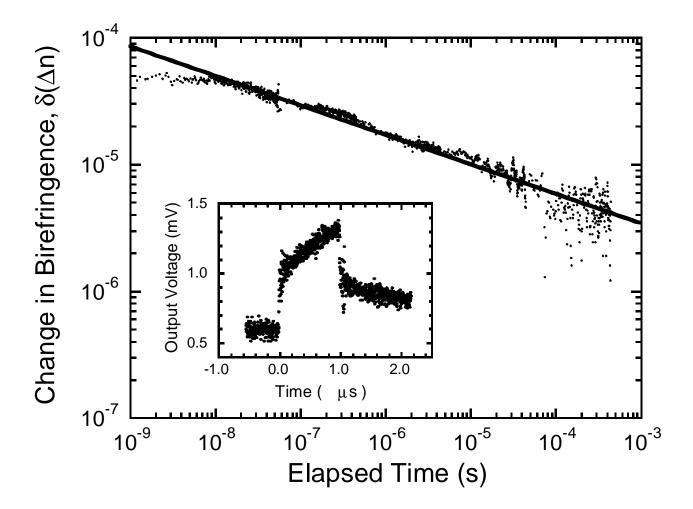
**Figure 1.** The change in birefringence of a KNbO<sub>3</sub> thin film after the removal of a 4 MV/m, 1  $\mu$ s electrical pulse. The data fit a power law (solid line) with an exponent  $m_{EO} = 0.2$ . The inset shows the measured response upon application and removal of the pulse on a linear scale.
