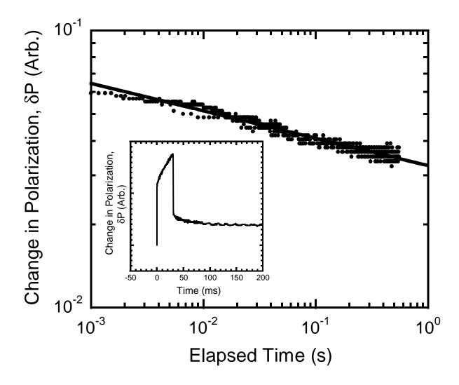
Figure 2. The change in the electronic polarization of a KNbO<sub>3</sub> thin film after the removal of a 1 MV/m, 30 ms electrical pulse. The data fit a power law (solid line) with an exponent,  $m_P = 0.1$ . The inset shows the data recorded during application and removal of the pulse on a linear scale.
