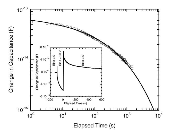
Figure 3. The relaxation of the change in capacitance at 1 MHz (1  $V_{pp}$ ) after removal of the bias field follows a modified stretched exponential as in Eq. 13 (solid line). The inset shows the capacitance before, during, and after application of a 4 MV/m bias for 100 s.
