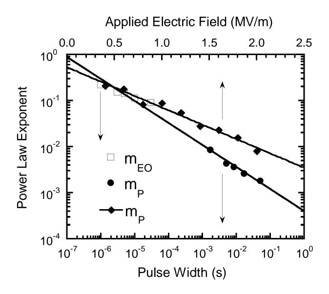
**Figure 4.** Dependence of the exponent  $m_{EO}$  ( ) on the duration of a 4 MV/m applied pulse and  $m_P$  (•) on the duration of a 2 MV/m applied pulse (lower x-axis). Also shown is the dependence of  $m_P$  (•) on the magnitude of a 2 ms applied pulse (upper x-axis). Lines are a guide to the eye.
