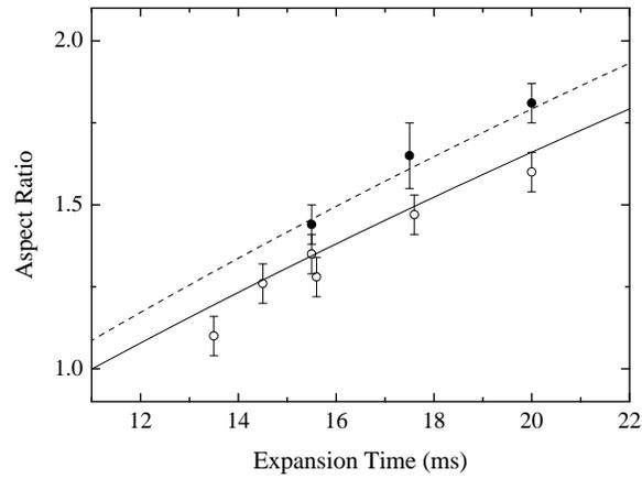
FIG. 4: Modification of the expansion of a Rb BEC due to interaction with the K Fermi gas. The radial-to-axial aspect ratio increases more rapidly with time for condensates created with K (solid circles) than for pure condensates (open circles). The two curves are the theoretical predictions for the expansion of a pure BEC for the trap parameters of the present experiment (solid line) and for trap frequencies 10% larger (dashed line).
