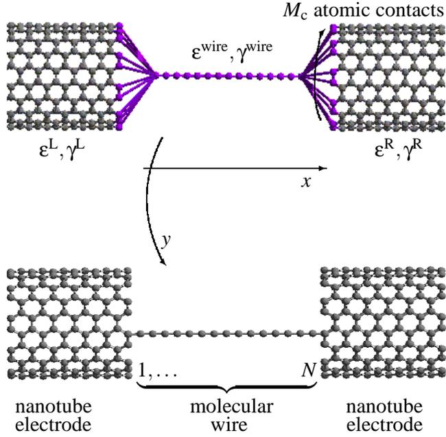
Fig. 1. Schematic representation of the molecular wire-carbon nanotube hybrid with single (bottom) and multiple (top) contacts. on-site energies  $\epsilon = \epsilon^L, \epsilon^R, \epsilon^{\text{wire}}$  are chosen to be zero.
