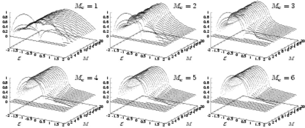
Fig. 3. The normalized spectral density  $\rho = \frac{2}{e}$  plotted for different maximum values  $M_c$  as in Fig. 2.; the x-axes represent the normalized energies  $\frac{2}{e} (E - \mu) = \frac{2}{e} E$ , the y-axes label the dimensionality of the leads (number of possible contacts)  $M_c$ .  $M_c \leq 20$  (a better resolution figure is available upon request).
