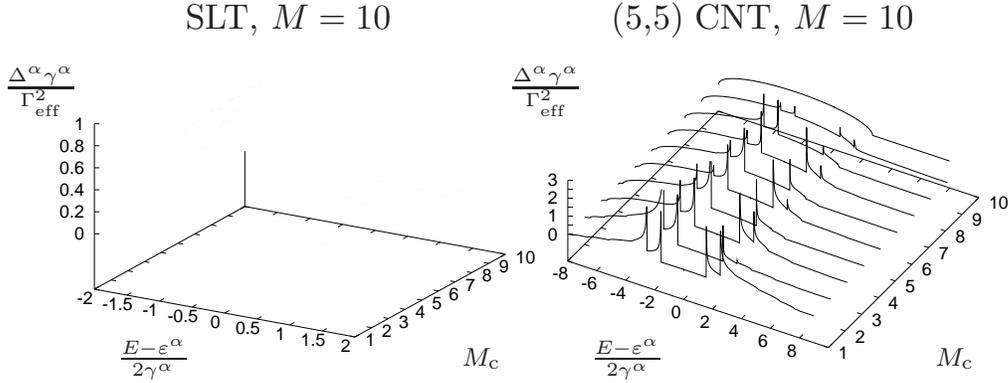
Fig. 5. The normalized spectral density as a function of energy and active contacts is plotted for  $M = 10$  possible atomic contacts available; on-site energies and hopping terms refer to  $\alpha = L; R$ -leads. The right panel illustrates numerical results after Ref. [42] in full agreement with the analytics showed in the text.
