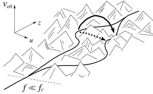
FIG. 1. Tunneling (lower dotted line) and activated motion (upper solid line) of an elastic string in a disordered potential under the action of a weak external force f \ll f_c .
