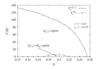
FIG. 1: has diagram for  $d_{x^2-y^2}$  and  $d_{x^2-y^2} + id_{xy}$  pairing in the HTCS. The parameters are appropriate for YBCO.
