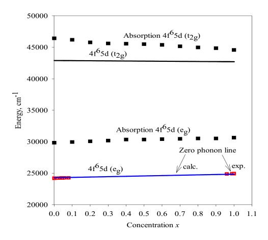
Figure 2:  $t_{2g}$  and  $\boldsymbol{e}_g$  levels of E  $\boldsymbol{u}^{2+}$  . Square sym bol refer to experim ent[2].
