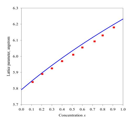
Figure 1: The lattice constant of S  $r_1\ _x B\ a_x F_2$  from  $\ x$  . Square symbol refer to experim ent [1].
