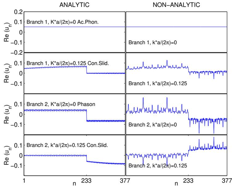
Figure 7: Lowest frequency modes in the double chain model. Same parameters as for Fig.4. The displacements are longitudinal and correspond to  $n = 1;233$  for the first chain and  $n = 234;377$  for the second chain. They are uniform for the acoustical phonon, antiparallel for the phason and practically involve only one of the two chains for concentrated sliding modes (the other chain presents only the small amplitude rapid oscillations equal to the derivative of the modulation function).
