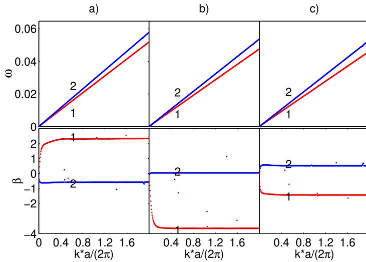
Figure 8: Unfolded dispersion curves and polarization parameters in the DCM model, when the single chain sound velocities  $v_i = a_i k^{(i)=m_i}$ ;  $i = 1;2$  are close one to another. a)  $v_1 = 0.9v_2$ ; b)  $v_1 = v_2$ ; c)  $v_1 = 1.1v_2$ ;
