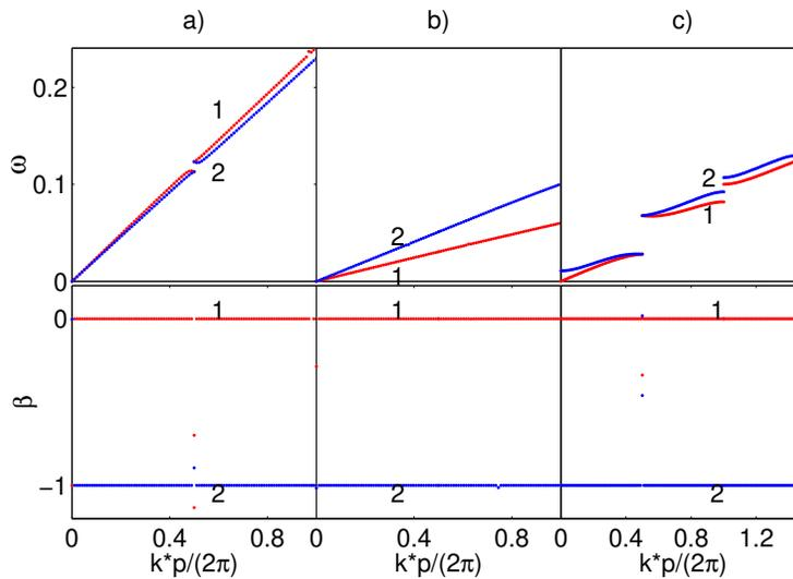
Figure 11: DIFFOUR model: Unfolded dispersion curves and polarization parameters. We used periodic boundary conditions  $pa_1 = qa_2$ . a)  $C = 0.4, A = 0.99A, B = 2.1C, p = 50; q = 17$ , analytic regime. b)  $C = 0.4, A = 0.99A, B = 2.5C, p = 50; q = 7$ , analytic regime. c)  $C = 0.4, A = 0.65A, B = 2.5C, p = 50; q = 7$ , non-analytic regime.
