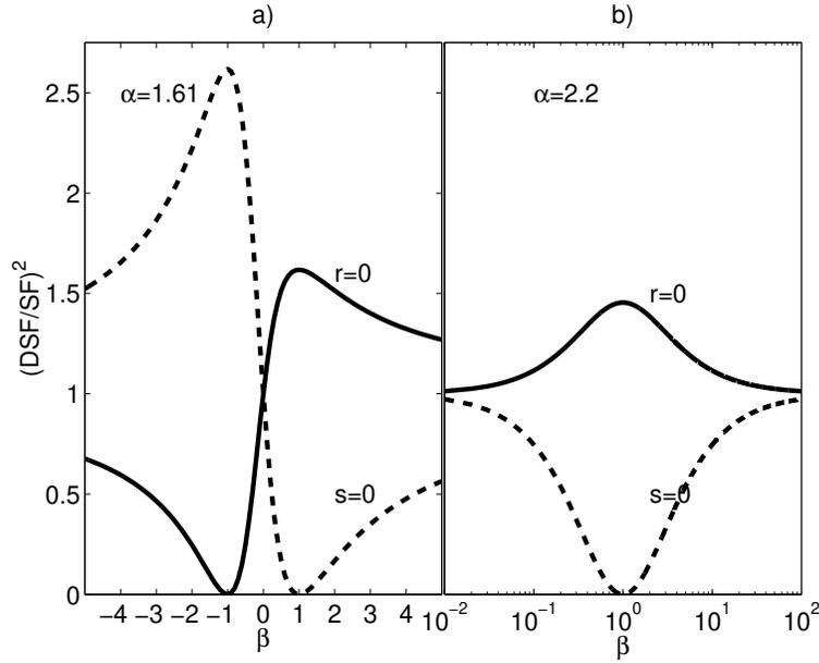
Figure 6:  $DSF/SF$  ratio for the main Bragg reflections of composites as a function of the inner polarization parameter of the mode. a) for  $\alpha = (1 + \sqrt{5})/2$ , as in Fig.4; b) for  $\alpha = 2/2$  as in the Bi 2212 lamellar superconductor.
