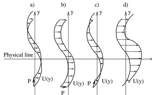
Figure 2: Different inner polarizations  $P$  and displacement hull function  $U$  for modulated crystals; a) phason with  $P \perp U$ , b) acoustical phonon  $P \parallel U$  ( $U$  is constant), c) mixed phonon/phason, d) distorted atomic surface, inner polarization can not be defined.
