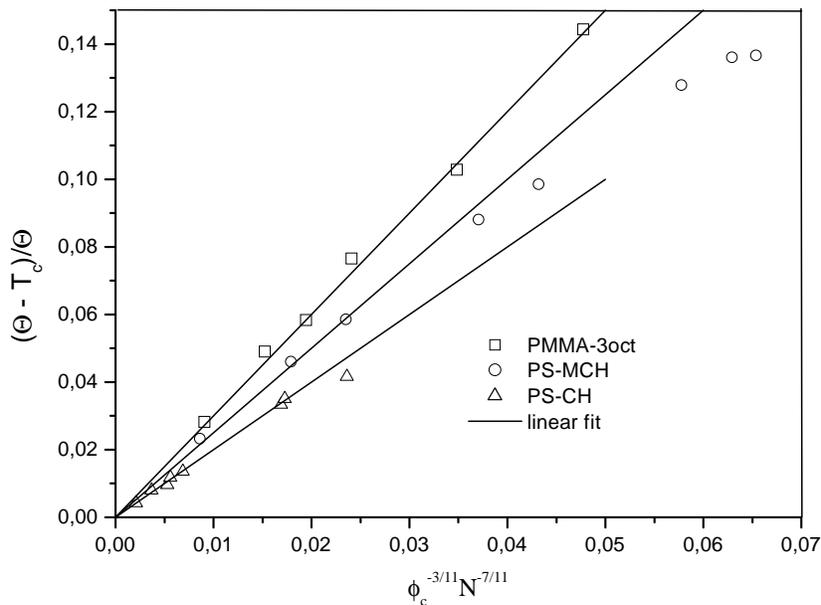
FIG. 7. The reduced temperature difference between the critical point and the  $\Theta$ -point is plotted versus  $\phi_c^{-3/11}N^{-7/11}$ . The symbols denote the critical parameter data for three experimental systems. The lines indicate the asymptotic linear approximation in accordance with Eq. (58).
