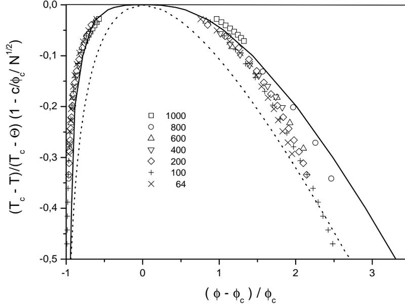
FIG. 9. Linear scaling plot of simulated phase-coexistence curves [49] for self-avoiding walks with nearest-neighbor interaction on a simple cubic lattice. The dotted curve represents the values calculated from the unrenormalized scaled free energy (29) and the solid curve represents the renormalized crossover theory with  $\bar{u} = 1$  and  $\tilde{c}_\rho = 1.5$ .
