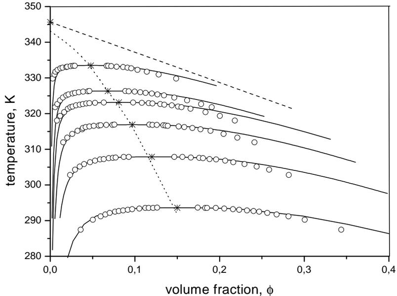
FIG. 4. Coexistence-curve data for PMMA in 3-octanone [46,47] are shown together with the result of the renormalized crossover theory. The dotted curve represents Eq. (59) with  $\Theta = 343.15$  K. The critical demixing points and the coexistence-curve scaling value of  $\Theta = 345.65$  K are denoted by stars. An estimate for the limiting phase-separation boundary with  $\phi_{sd}/\phi_c = 3$  is shown by the dashed line.
