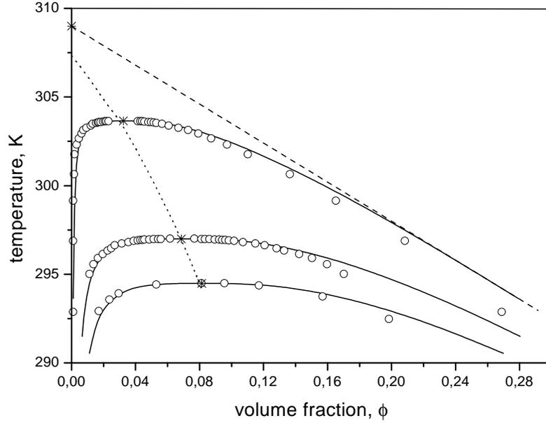
FIG. 2. Coexistence-curve data for PS in cyclohexane [42–44] are shown together with the result of the renormalized crossover theory (full curves). The dotted curve represents Eq. (59) with  $\Theta = 307.25$  K. The critical demixing points and the coexistence-curve scaling value of  $\Theta = 309$  K are denoted by stars. An estimate for the limiting phase-separation boundary with  $\phi_{sd}/\phi_c = 3$  is shown by the dashed line.
