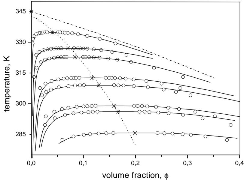
FIG. 3. Coexistence-curve data for PS in methylcyclohexane [45] are shown together with the result of the renormalized crossover theory (full curves). The dotted curve represents Eq. (59) with  $\Theta = 342.75$  K. The critical demixing points and the coexistence-curve scaling value of  $\Theta = 345$  K are denoted by stars. An estimate for the limiting phase-separation boundary with  $\phi_{sd}/\phi_c = 3$  is shown by the dashed line.
