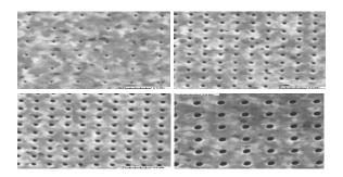
FIG.1. Focused ion beam m illed arrays of cylindrical pinholes in a 400 nm thick free standing gold  $\,$  lm. The scale bar is 500 nm.
