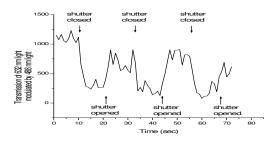
FIG.3. M odulation of the 20 nm pinholes array transm ission at 633 nm induced by m odulation of control light. The shutter of control light was closed and opened three times during the experiment.
